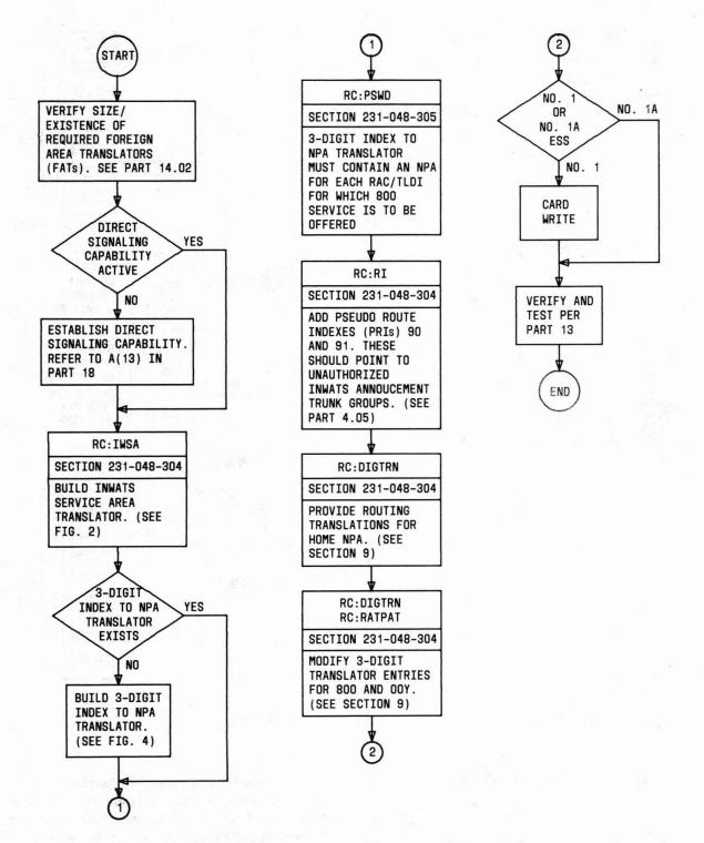
Fig. 9—Establishing 800 Service in an OSO
