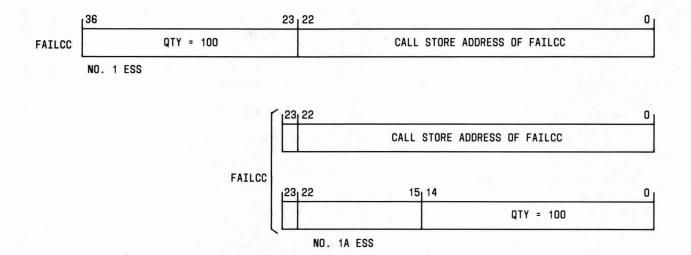
FAILCC = CCIS INWATS FAILURE CODE CONTROL TABLE
