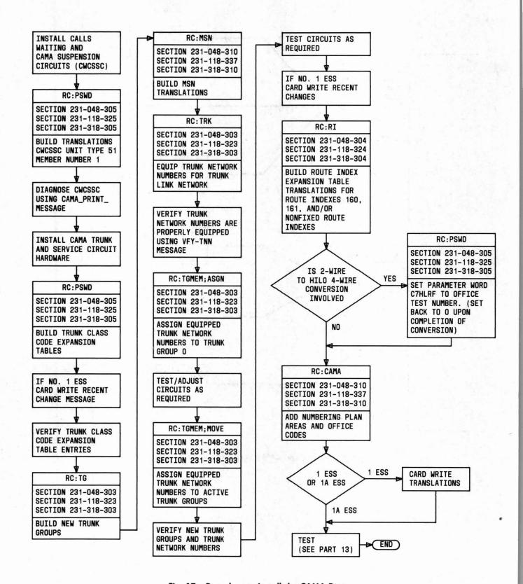
Fig. 17—Procedure to Install the CAMA Feature
