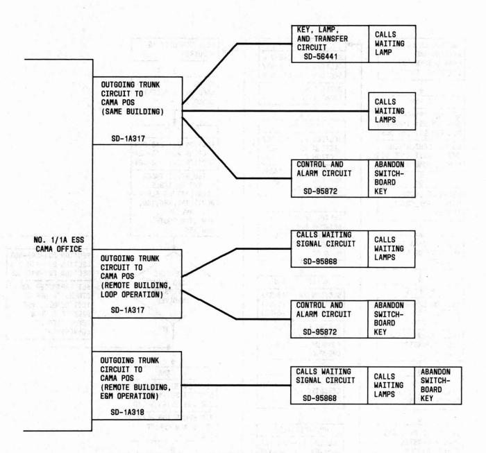
Fig. 18—Calls Waiting and CAMA Suspension Circuit Arrangement
