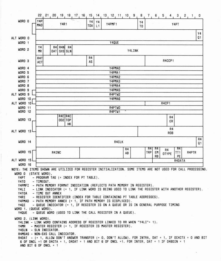
Fig. 3—DAL Ringing Register Layout (Sheet 1)
