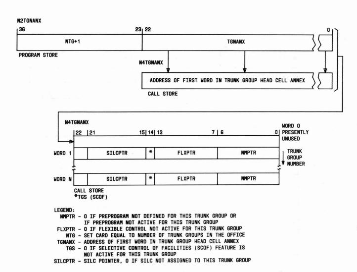
Fig. 24—Trunk Group Head Cell Annex Layout and Parameter Word N2TGNANX
