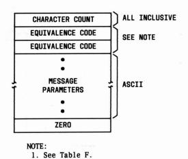
Fig. 43—EADAS/NM Input Message Format
