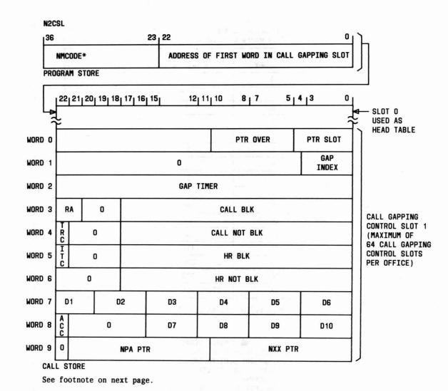
Fig. 22—Call Gapping Control Slot Layout—N2CSL (Sheet 1 of 2)
