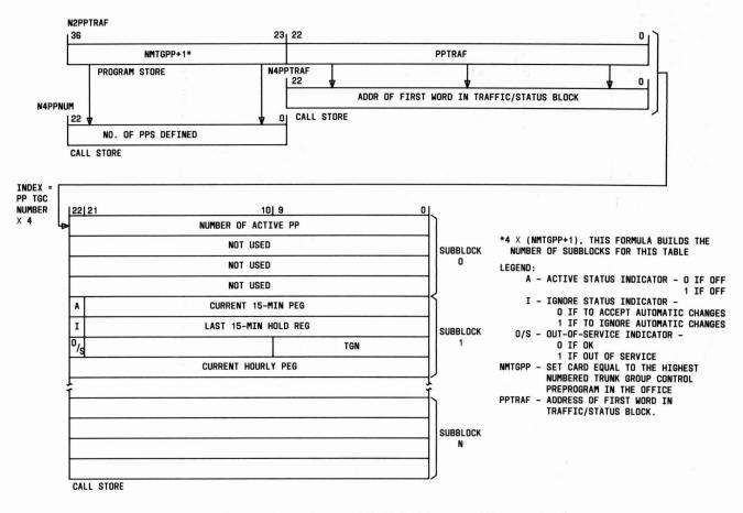
Fig. 26—Trunk Group Control Status and Traffic Block Layout and Parameter Word N2PPTRAF
