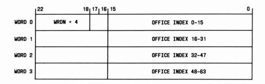
Fig. 19—MEMN 10 Through 17 Auxiliary Block
