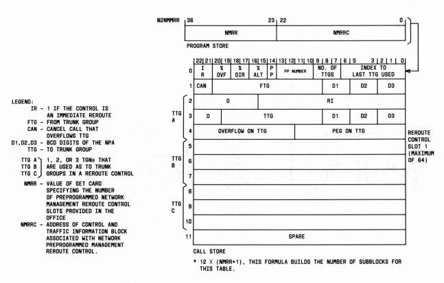
Fig. 42—Network Management Reroute Control Slot Layout
