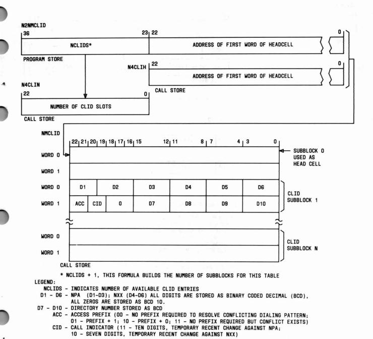
Fig. 23—CLID Control Slot Layout
