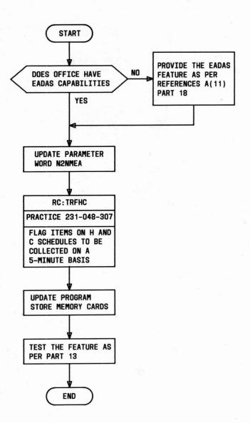
Fig. 93—Growth/Retrofit Procedures for Operation With EADAS/NM
