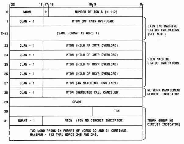
In the 4-wire network, these indicators are machine congestion level 1 for MF and DP receivers and machine congestion level 2 for MF and DP receivers.
