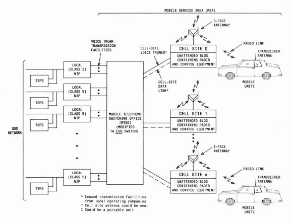
Fig. 1 — Primary System Interfaced to DDD Network
