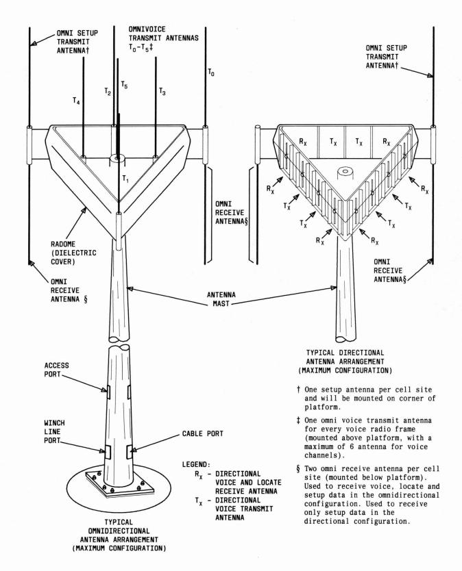
Fig. 26 — Cell Site Antenna Configurations
