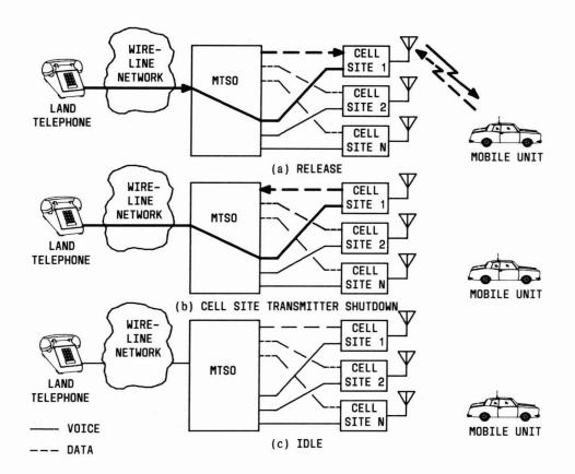
Fig. 9 — Disconnect Sequence (System Initiated)
