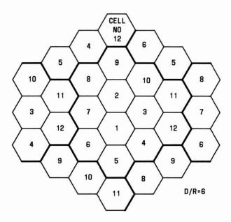
Fig. 13 — Cell Reuse Pattern for Start-Up Configuration
