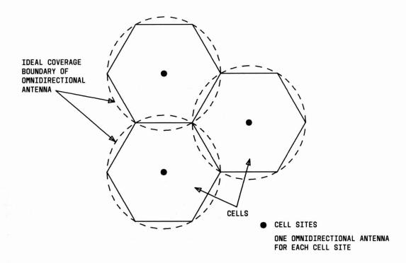
Fig. 12 — Cells Served by Omnidirectional Antennas
