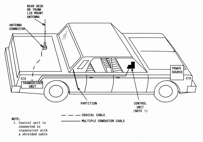
Fig. 19 — Typical Mobile Unit Equipment Placements and Connections
