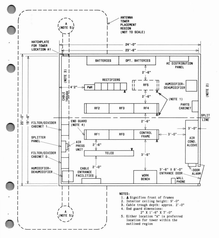
Fig. 23 — Typical Cell Site Equipment Configuration
