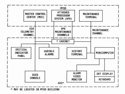
Fig. 3 — ACC/MTSO Channel Interface
