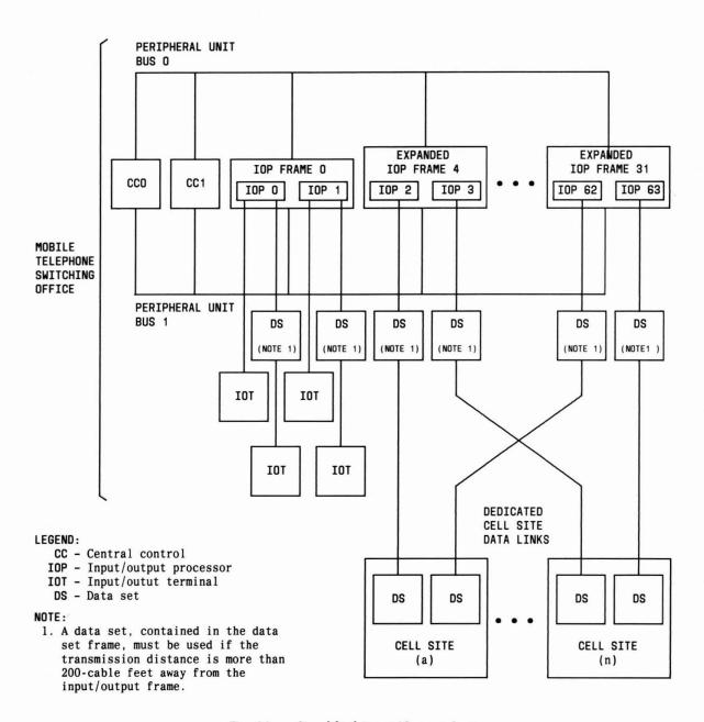
Fig. 32 — Simplified Input/Output System
