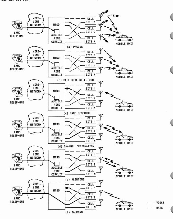
Fig. 5 — Mobile-Completed Call Sequence
