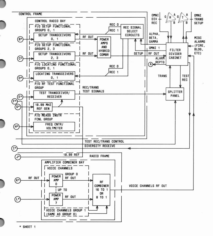
Fig. 22 — Cell Site Functional Block Diagram (Sheet 2 of 2)
