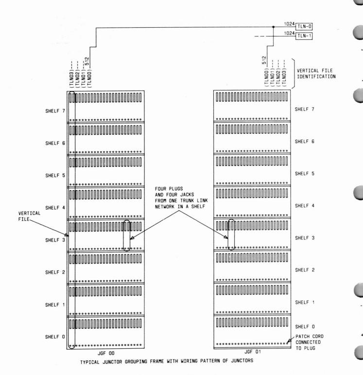
Fig. 36 — JGF Layout - 12 Vertical File
