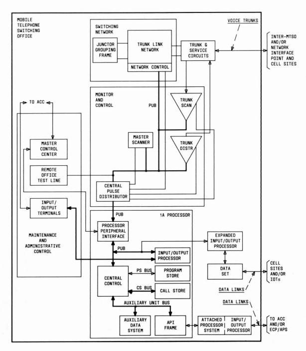
Fig. 27 — MTSO Equipment Interconnections Block Diagram
