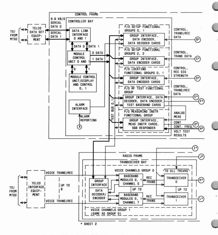
Fig. 22 — Cell Site Functional Block Diagram (Sheet 1 of 2)
