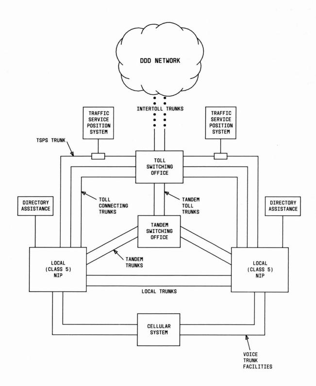
Fig. 2 — Switching Hierarchy Block Diagram
