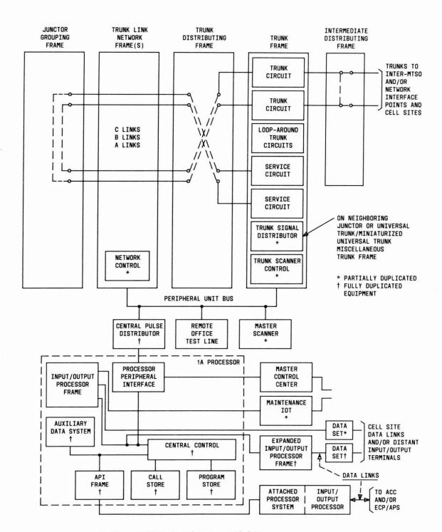
Fig. 37 — MTSO Duplicated Equipment Block Diagram
