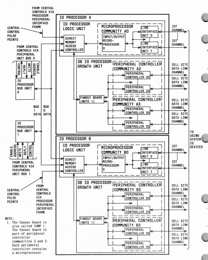
Fig. 31 — IOP Frame Block Diagram (Equipped with 3B IOP Growth Units)
