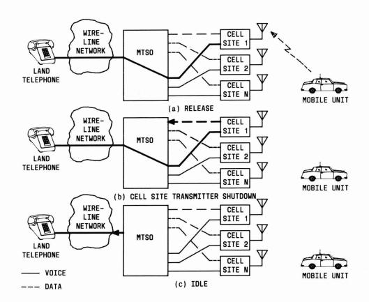
Fig. 8 — Disconnect Sequence (Mobile Initiated)
