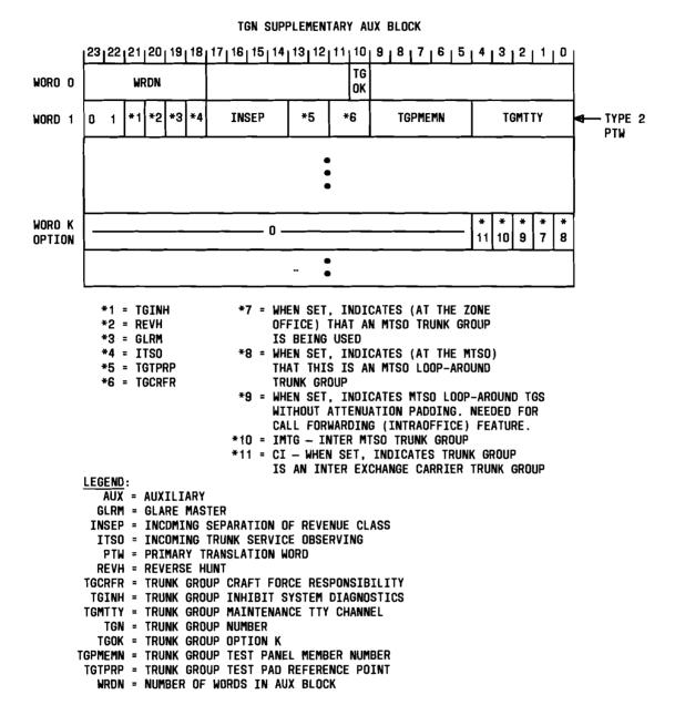
Fig. 9 — TGN Supplementary Auxiliary Block
