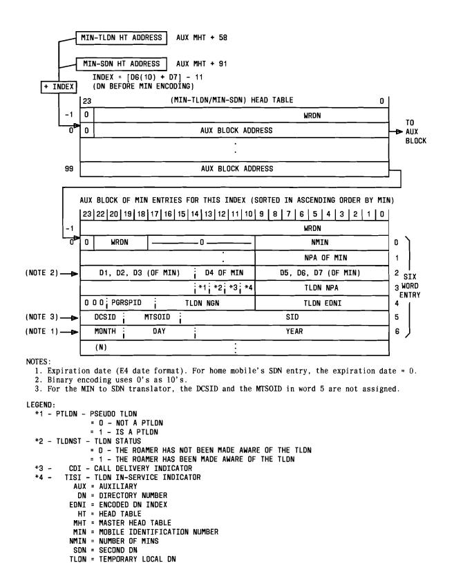
Fig. 24 — MIN-TLDN and MIN-SDN Translators
