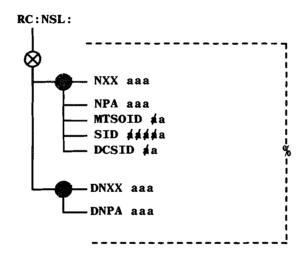
Fig. 54 — Building the Network Service List (RC:NSL)
