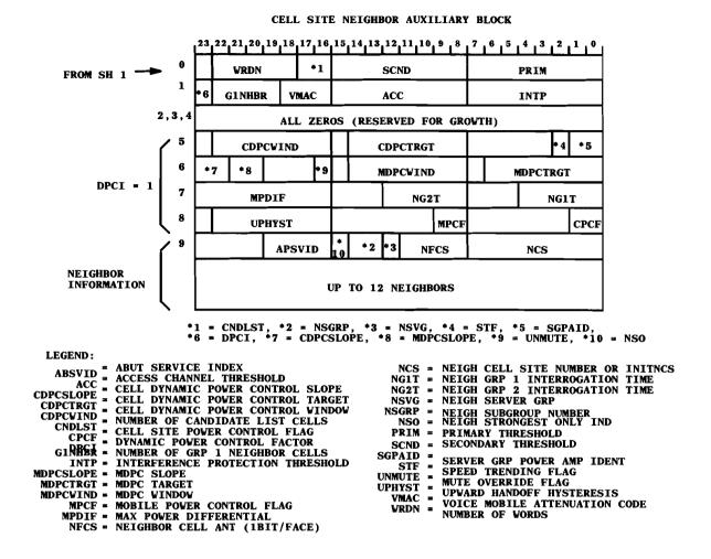
Fig. 23 — Cell Master Location Translator (Sheet 2 of 2)
