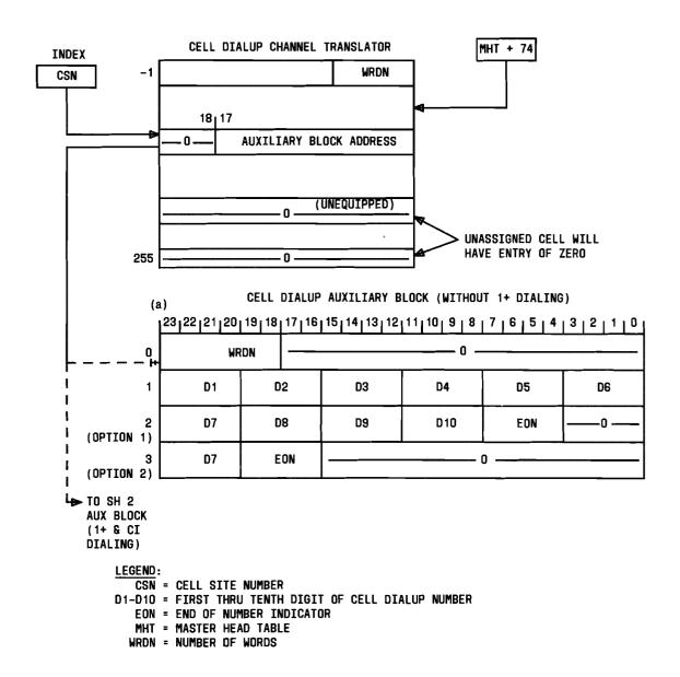
Fig. 17 — Cell Dialup Channel Translator (Sheet 1 of 2)
