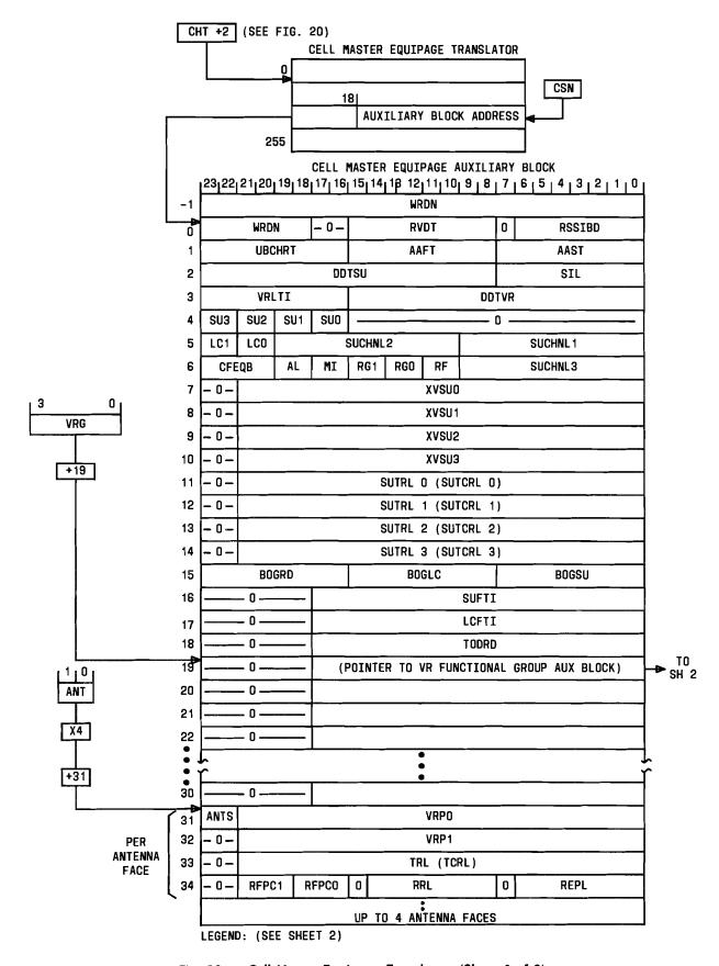
Fig. 22 — Cell Master Equipage Translator (Sheet 1 of 2)
