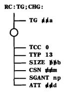
Fig. 31 — Changing a Trunk Group to a Cell Site (RC:TG;CHG)
