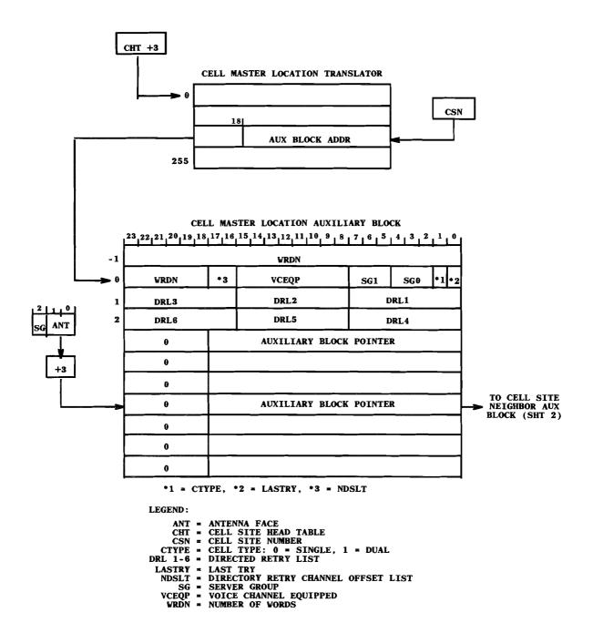
Fig. 23 — Cell Master Location Translator (Sheet 1 of 2)
