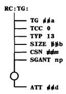
Fig. 30 — Adding a Trunk Group to a Cell Site (RC:TG)
