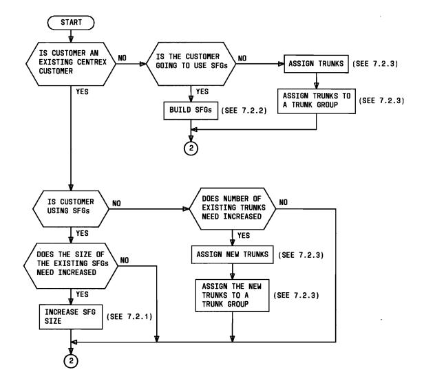
Fig. 12 — CWC Access to Private Facilities Implementation Sequence Flow Diagram (Main Location Only) (Sheet 1 of 3)
