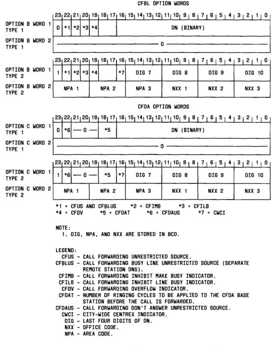
Fig. 9 — MLHG Auxiliary Block - CFBL/CFDA Option Words
