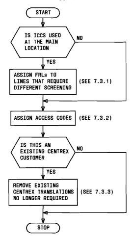
Fig. 14 — CWC Access to Private Facilities Implementation Sequence Flow Diagram (Remote Location Only)
