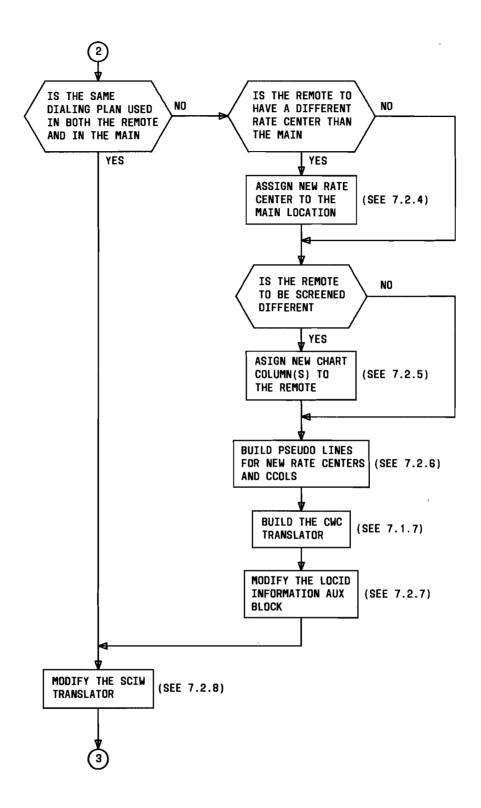
Fig. 12 — CWC Access to Private Facilities Implementation Sequence Flow Diagram (Main Location Only) (Sheet 2 of 3)
