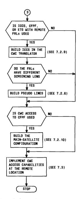
Fig. 12 — CWC Access to Private Facilities Implementation Sequence Flow Diagram (Main Location Only) (Sheet 3 of 3)
