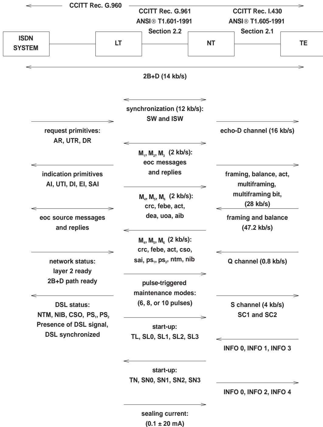
Figure 2.2.3-6 — ISDN Basic Access Signals
