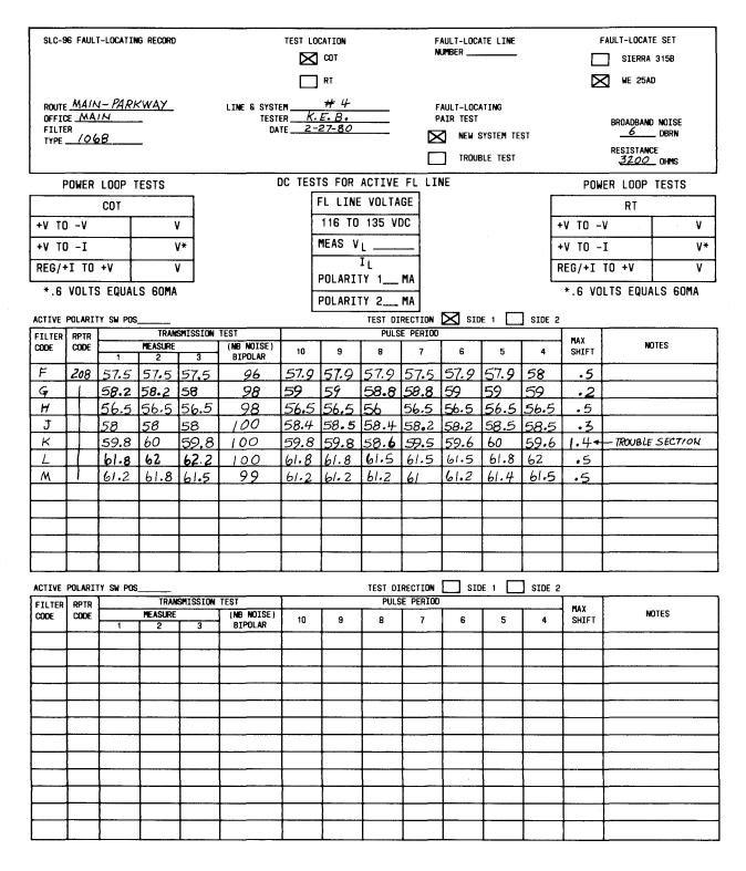
Fig. 16—Results of a Digital Line With Marginal Trouble Using the 25AD
