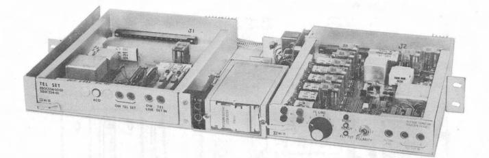
Fig. 5—COT Fault-Locate and Order Wire Panel (J1C141AC-L1)
