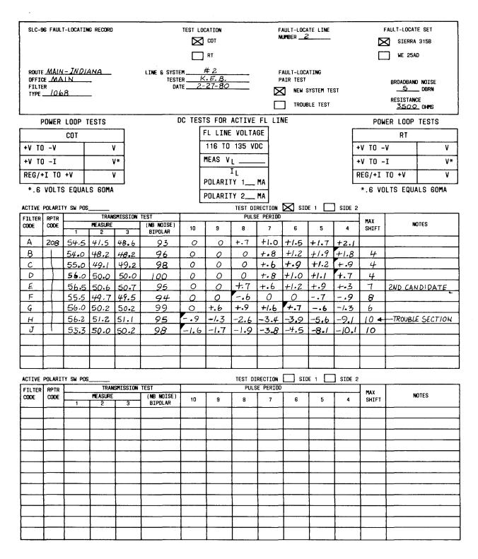
Fig. 14—Results of a Digital Line With Marginal Trouble Using the 315B
