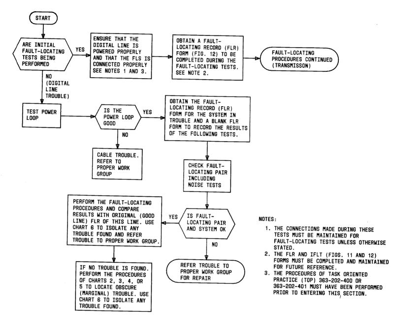
Fig. 1—SLC-96 Fault-Locating Sequence Chart
