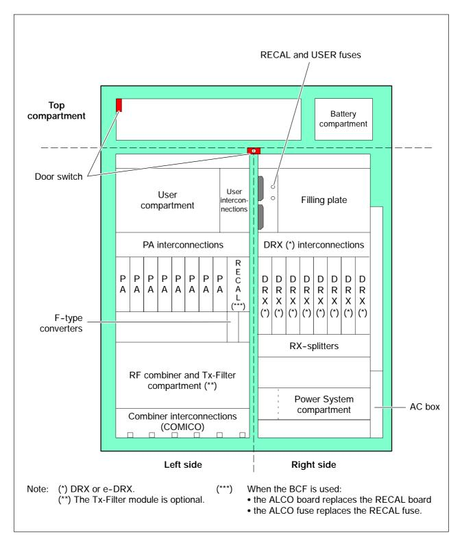
Figure 3-46 S8000 Outdoor BTS: Extension cabinet layout
