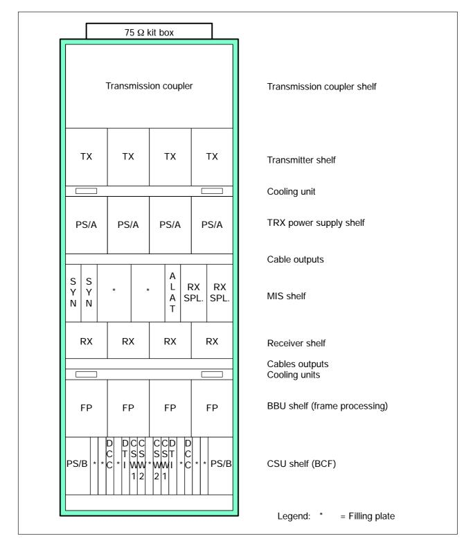
Figure 3-35 S4000C BTS: Base cabinet (2S323 configuration)
