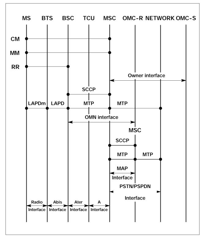
Figure 1-3 Radio cellular system interfaces
