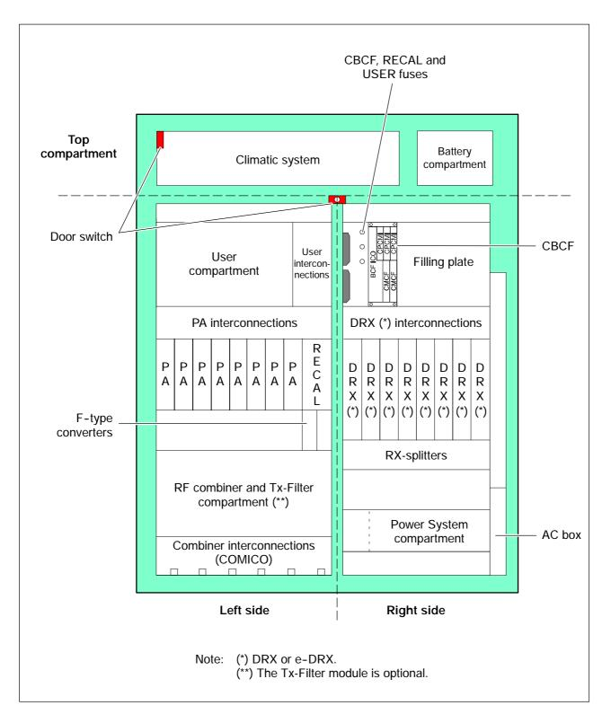
Figure 3-45 S8000 Outdoor BTS: Base cabinet layout (with CBCF Module)
