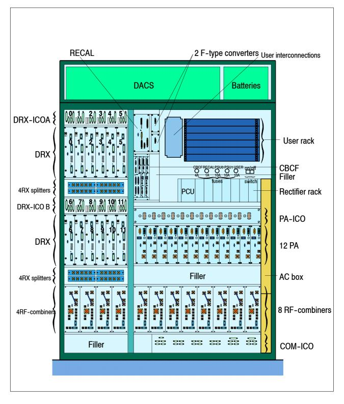
Figure 3-51 S12000 Outdoor BTS: Base cabinet inside view
