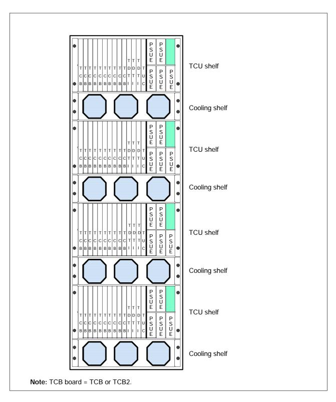
Figure 5-5 TCU cabinet (fully equipped)
