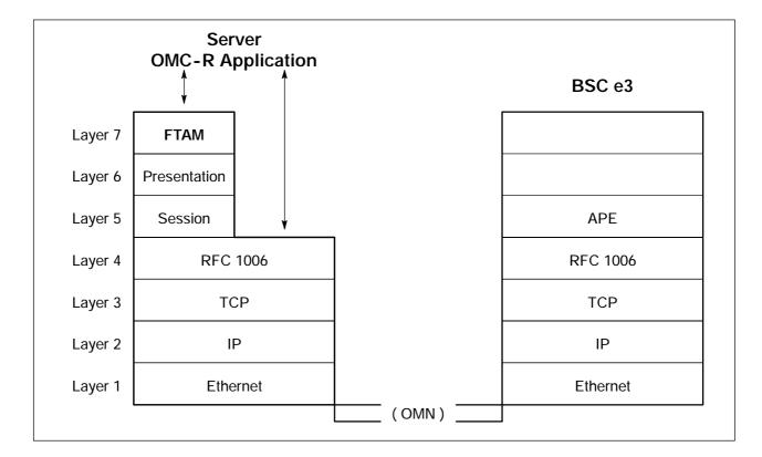
*Figure 8-10* shows the TCP/IP protocols used for the server.
