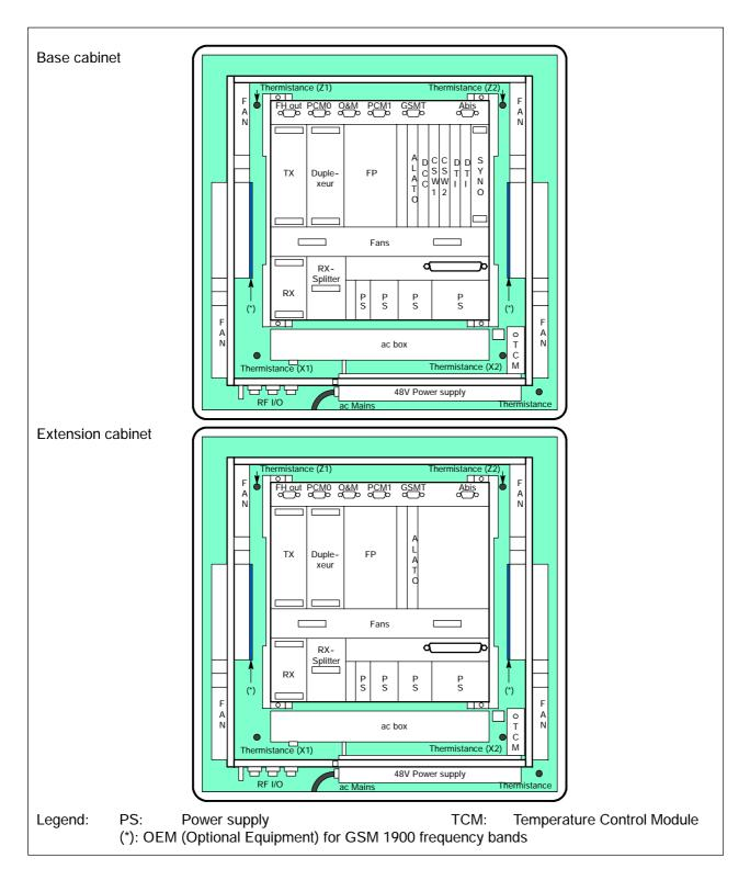
Figure 3-24 S2000E Outdoor BTS: Base and extension cabinets front panels
