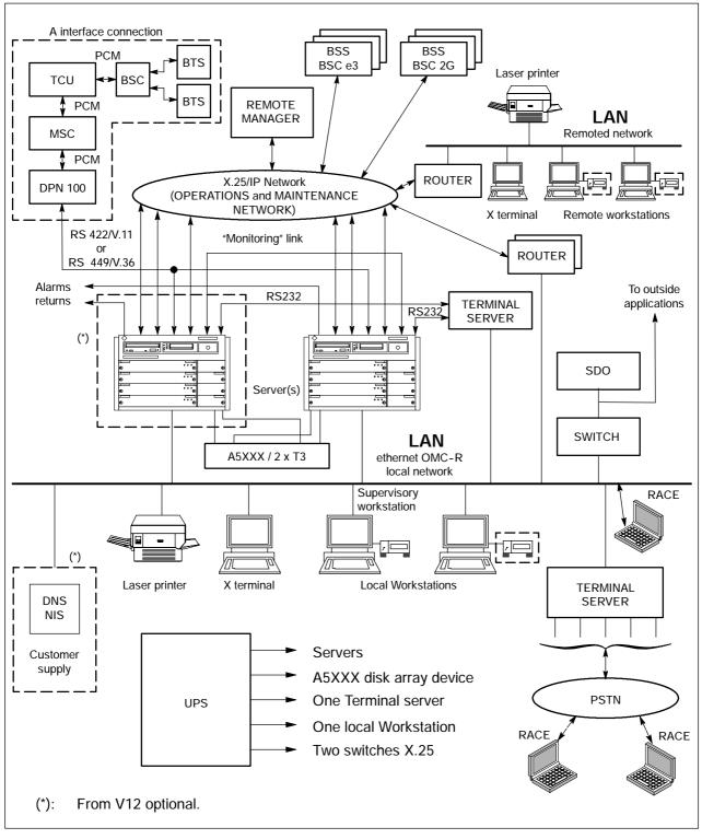
Figure 7-3 Physical architecture of the OMC-R (Server E4XXX and A5XXX) remote operation in line mode via terminal server
