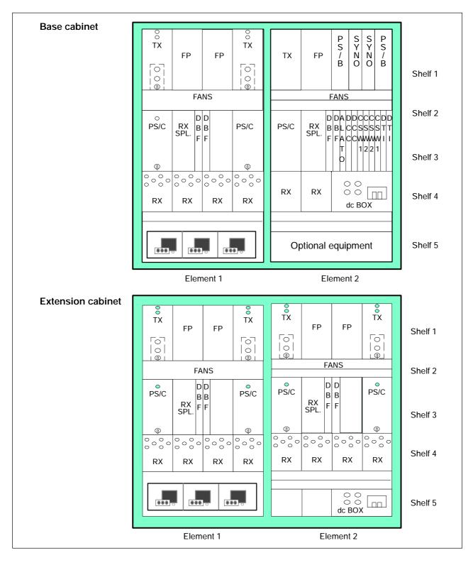
Figure 3-40 S4000 Smart BTS: Base and extension cabinets
