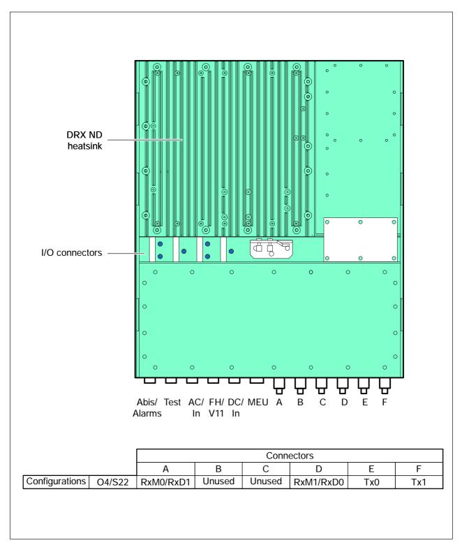
Figure 3-29 S2000H "EP" BTS: Extension unit
