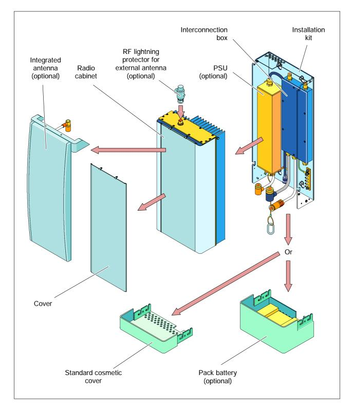
Figure 3-32 e-cell part assembly
