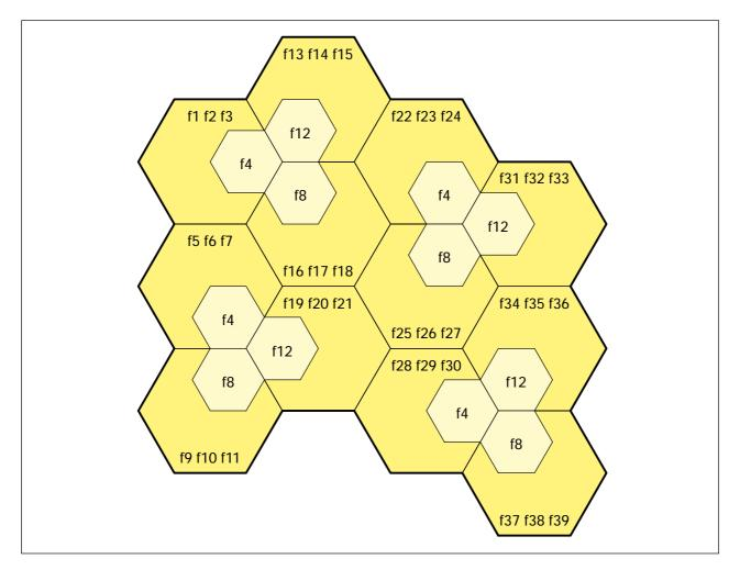
Figure 2-4 Concentric-cell network
