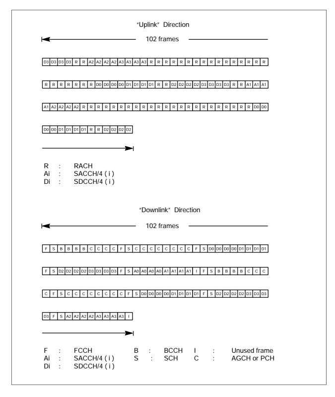
Figure 8-5 Logical channel multiplexing onto a combined BCCH channel
