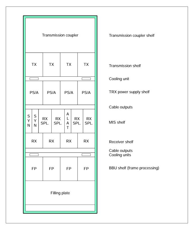
Figure 3-36 S4000C BTS: Extension cabinet (2S323 configuration)
