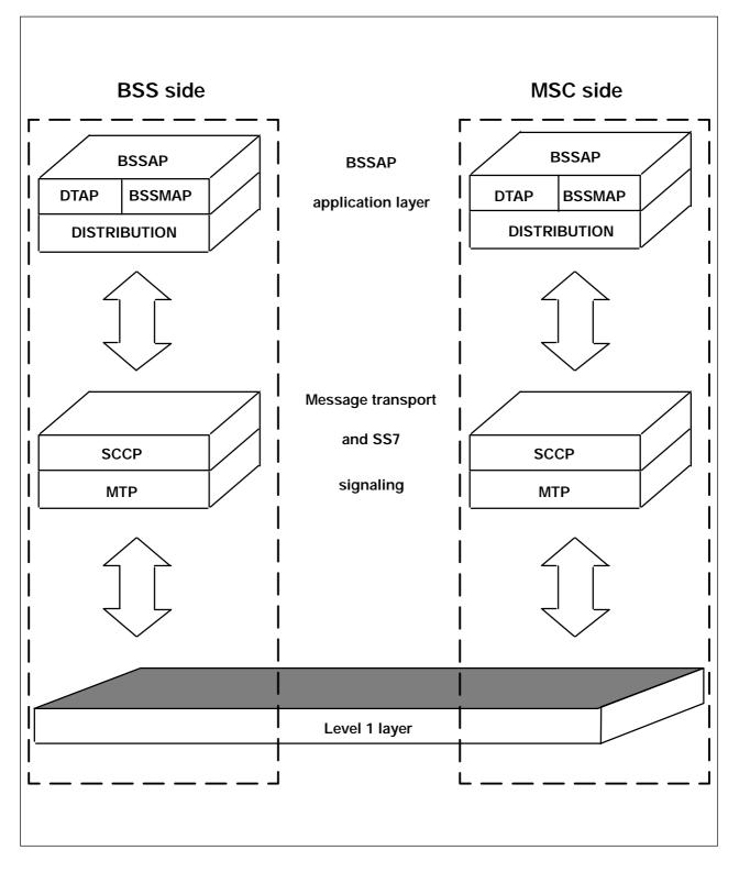
Figure 8-9 Architecture of the A-interface
