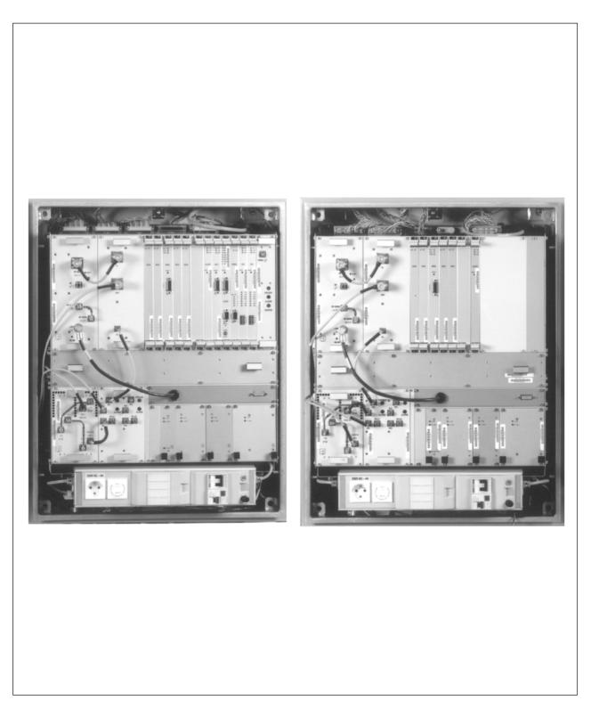
Figure 3-2 S2000E Indoor BTS: Base and extension cabinets (inside view)
