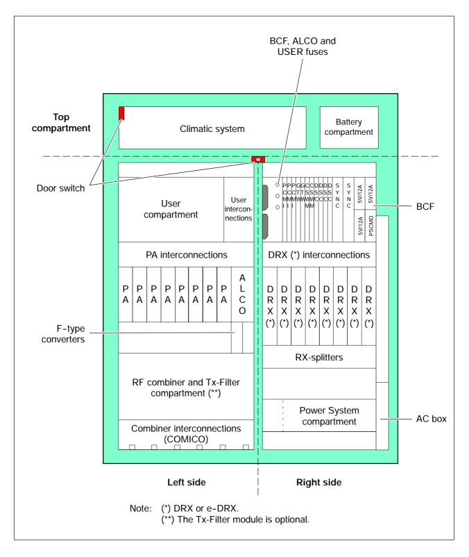
Figure 3-44 S8000 Outdoor BTS: Base cabinet layout (with BCF unit)
