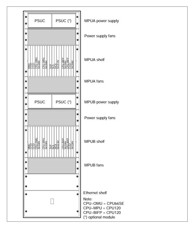
Figure 4-6 Fully equipped BSC 12000 control cabinet
