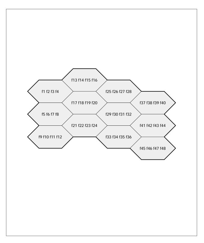
Figure 2-7 Non concentric-cell network
