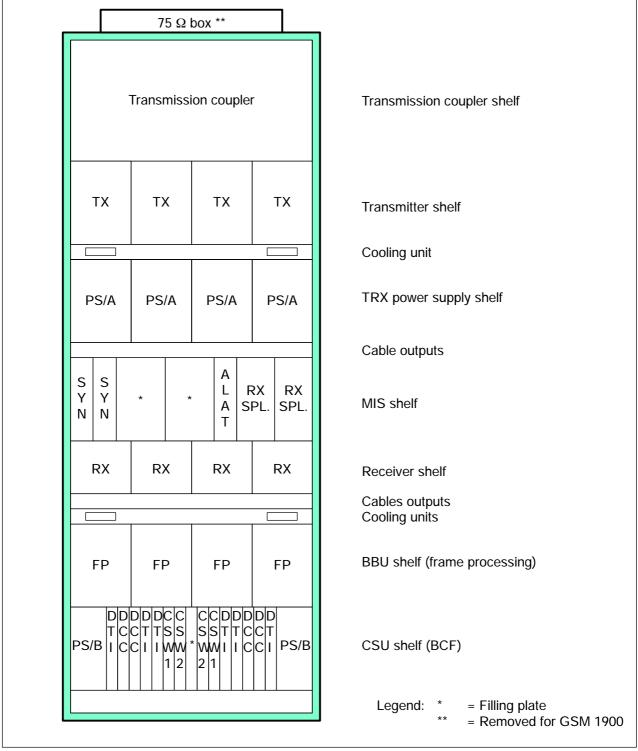
Figure 3-33 S4000 Indoor BTS: Base cabinet (fully equipped with diversity)
