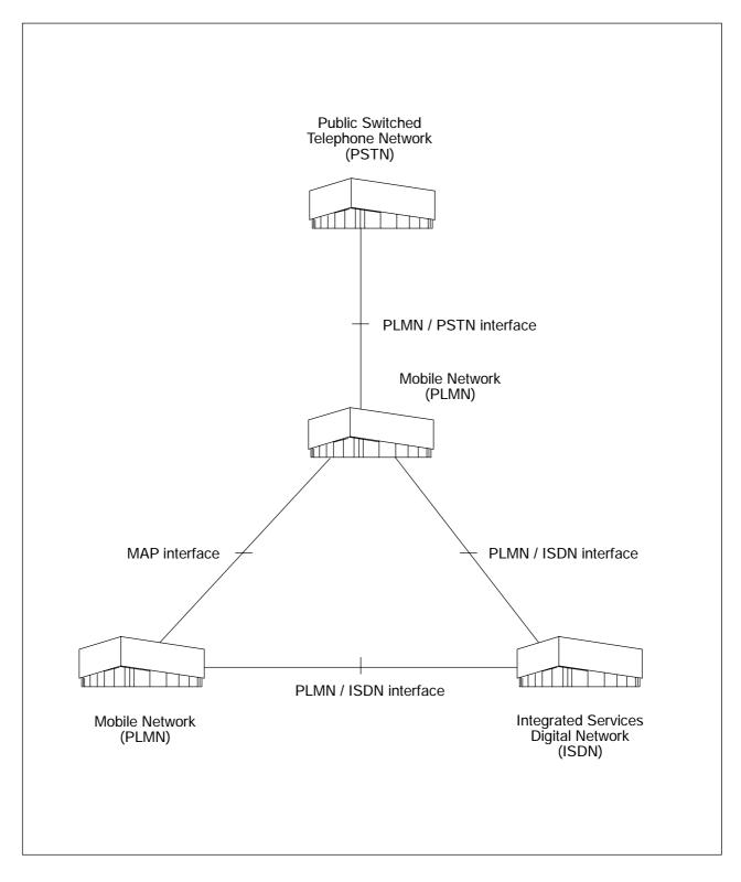
Figure 8-13 Connections between networks
