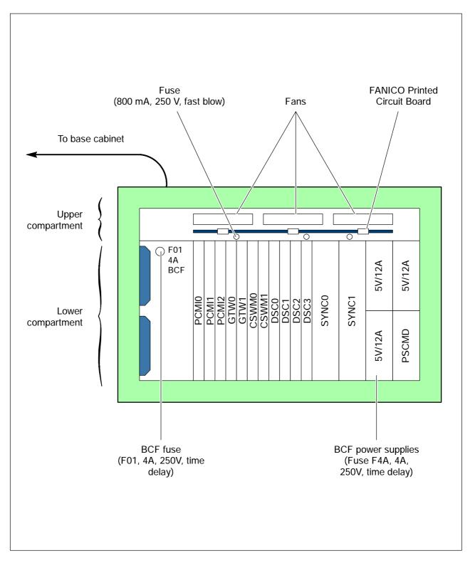
Figure 3-43 S8000 Indoor BTS: BCF cabinet layout
