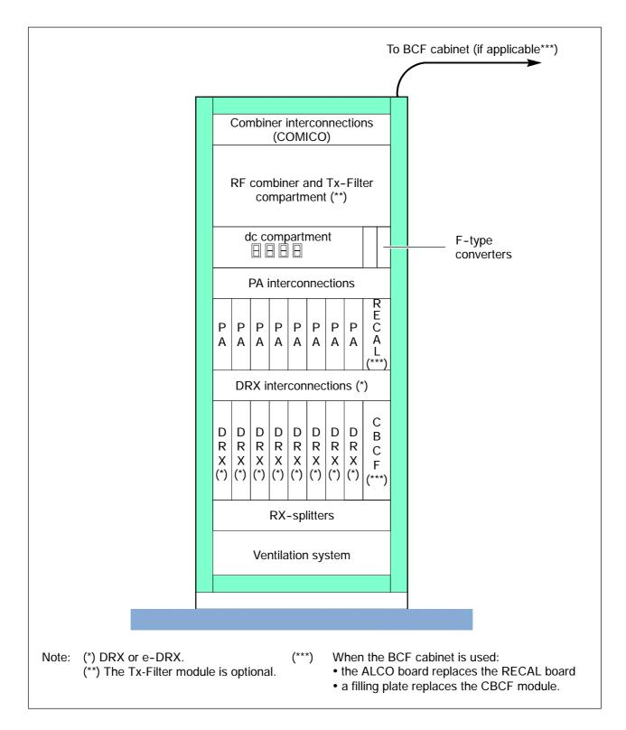
Figure 3-42 S8000 Indoor BTS: Base cabinet inside view
