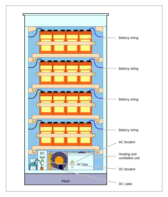
Figure 3-54 Battery Cabinet (type 3)
