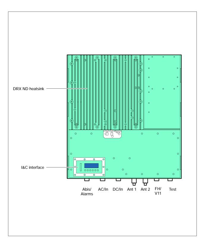
Figure 3-30 S2000L "EP" BTS: Base unit
