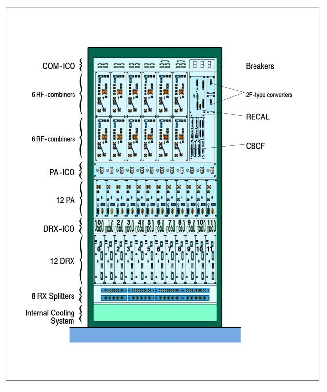
Figure 3-50 S12000 Indoor BTS: Base cabinet inside view
