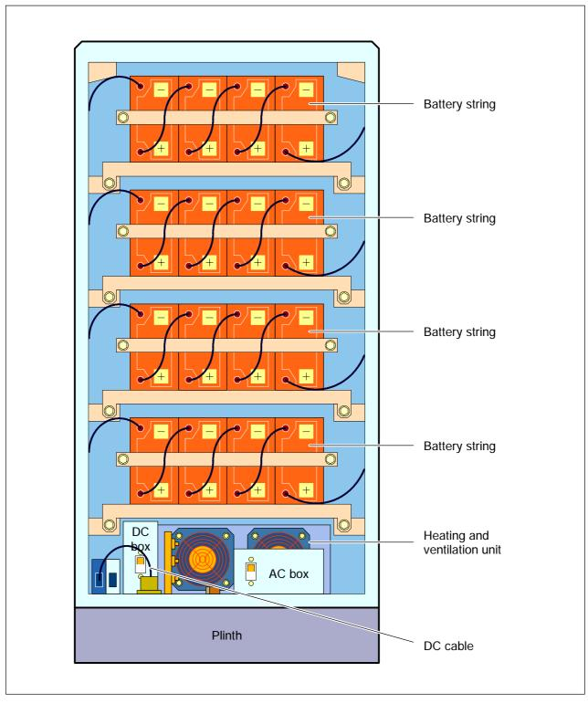
Figure 3-53 Battery cabinet (type 2)
