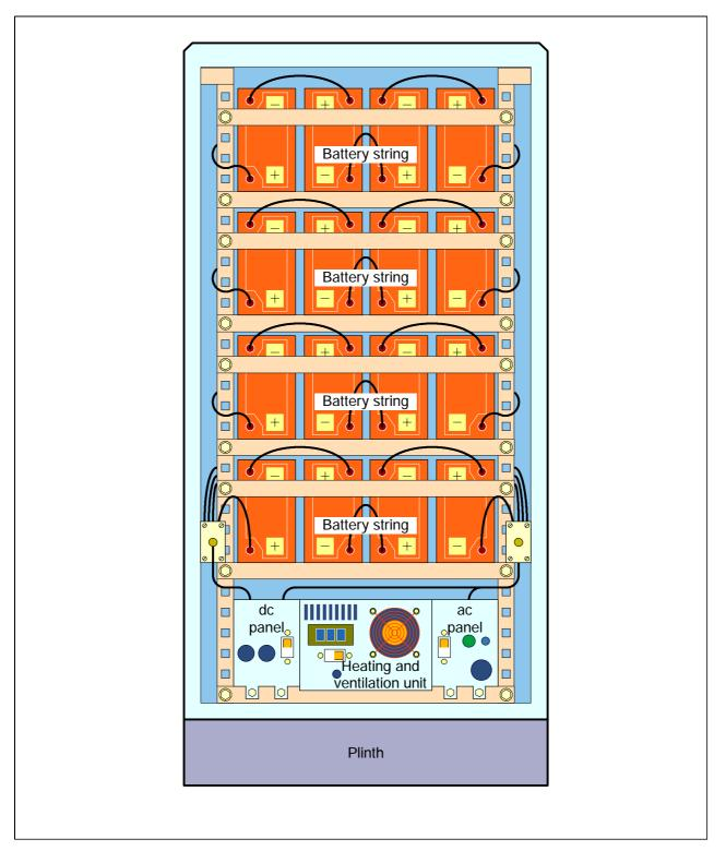
Figure 3-52 Battery cabinet (type 1)
