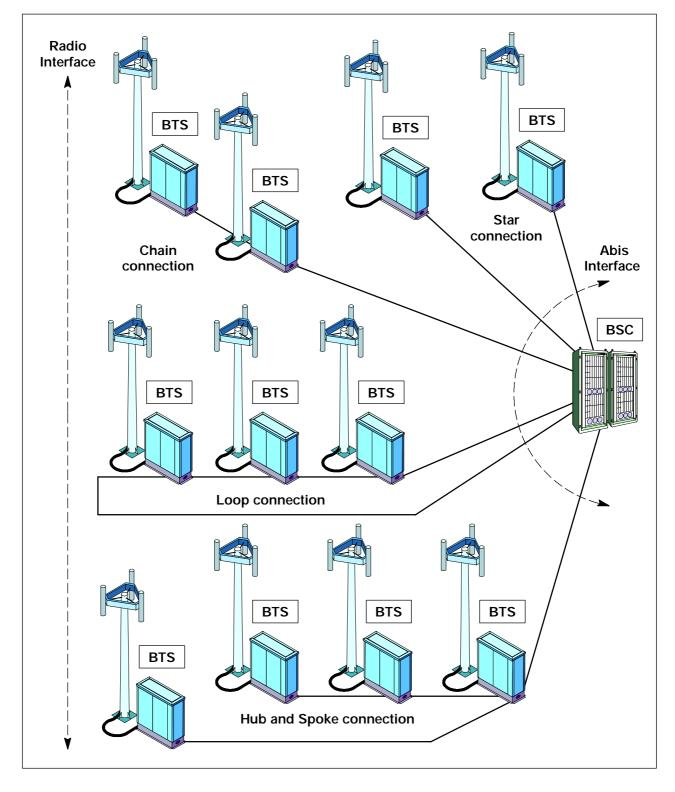
Figure 3-22 Examples of BTS connections
