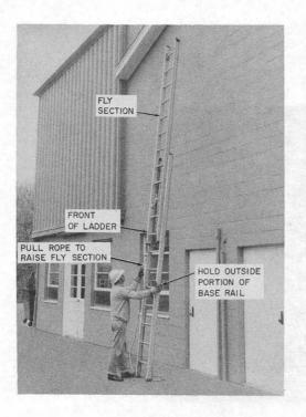
Fig. 24—Fly Section Extended
