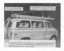
Fig. 4-Mounting Ladder on Roof-Type Ladder Bracket
