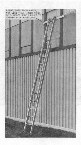
Fig. 16—Ladder Placed in Front of Window
