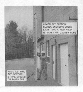
Fig. 26-Fly Section Lowered
