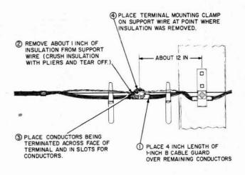
Fig. 10—Attaching 105A Wire Terminal
