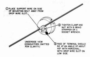
Fig. 11—Attaching Support Wire
