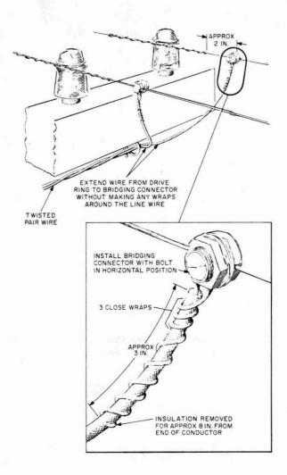
Fig. 7—Where Line Wires are Tied to Pin-Type
