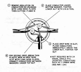
Fig. 12—Terminating Wire Leads
