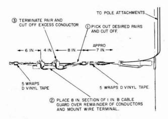
Fig. 15—Location of Wire Terminals at Dead-End Pole
