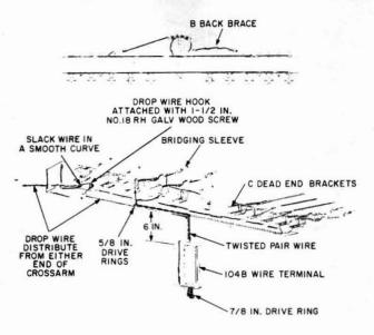
Fig. 4—For More Than Two Drops Use a 104B Wire Terminal Mounted on Pole
