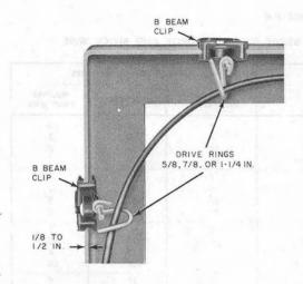
Fig. 18—B Beam Clips
