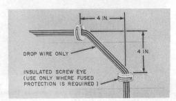
Fig. 17—Spacing Insulated Screw Eye When Changing Direction of Wire Run
