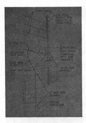
Fig. 10-Drop Wire Attached to Power Fixture
