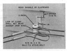
Fig. 6—First Attachment, House Bracket Horizontal
