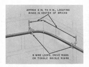
Fig. 16—Spacing Attachments at Inside Corner of Building
