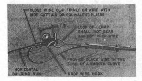
Fig. 3—First Attachment, Drop Wire Hook
