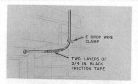
Fig. 19—Last Attachment, Building Entrance Slopes
