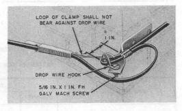
Fig. 7—First Attachment, Corner Bracket
