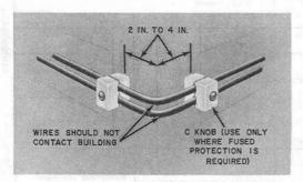
Fig. 15—Spacing C Knobs on Outside Corner of Building
