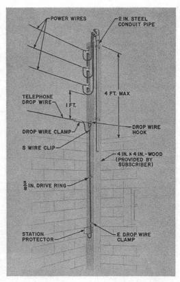
Fig. 13—Drop Wire Attached to Subscriber Pole
