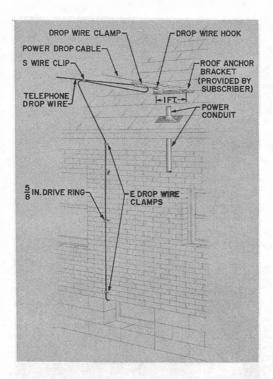
Fig. 12—Drop Wire Attached to Roof Anchor Bracke
