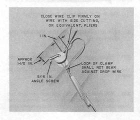
Fig. 1-First Attachment, Horizontal Run
