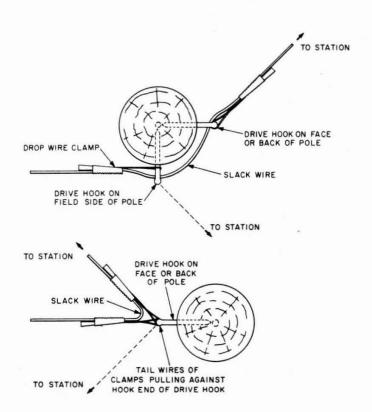
Fig. 5—Distributing Wires From Pole Other Than
