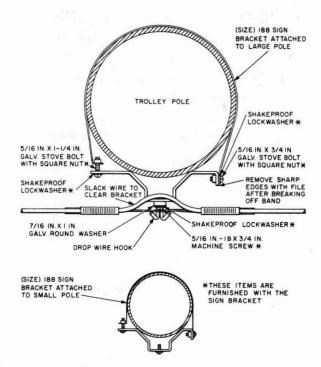
Fig. 8—Attachment to Type 188 Sign Bracket
