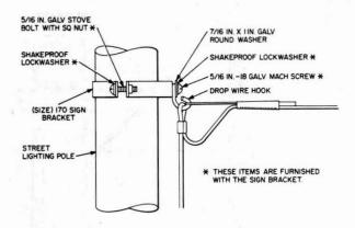
Fig. 7—Attachment to Type 170 Sign Bracket
