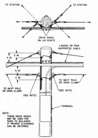
Fig. 2—Terminal Mounted on Cable Side of Pole
