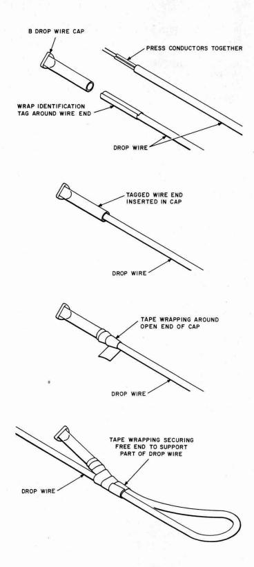
Fig. 3—Disposition of Disconnected Drop Wire
