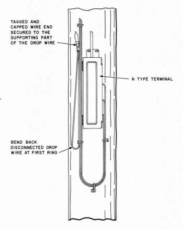
Fig. 4—N-Type Terminal, Pole Mounted
