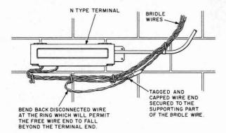
Fig. 6-N-Type Terminal Wall Mounted
