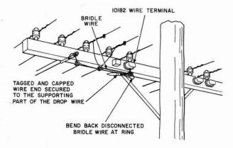
Fig. 8—Wire Terminal Mounted on Crossarm
