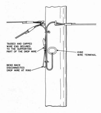
Fig. 7—101-Type Wire Terminal, Pole Mounted
