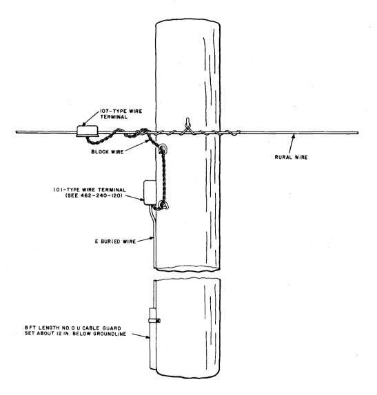
Fig. 30—Termination of E Buried Wire and Rural Wire
