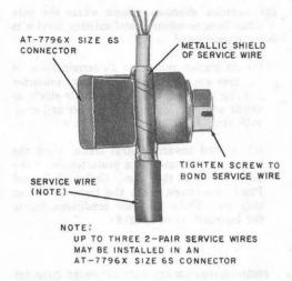
Fig. 4-DService Wire Installed in AT-7796X Connector
