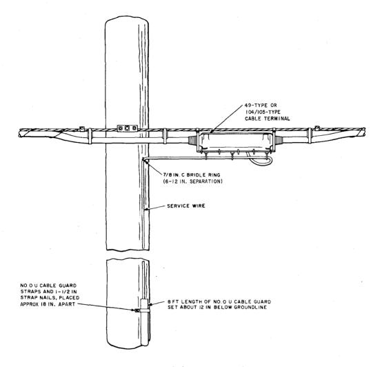
Fig. 25—Buried Plant Run Up a Pole
