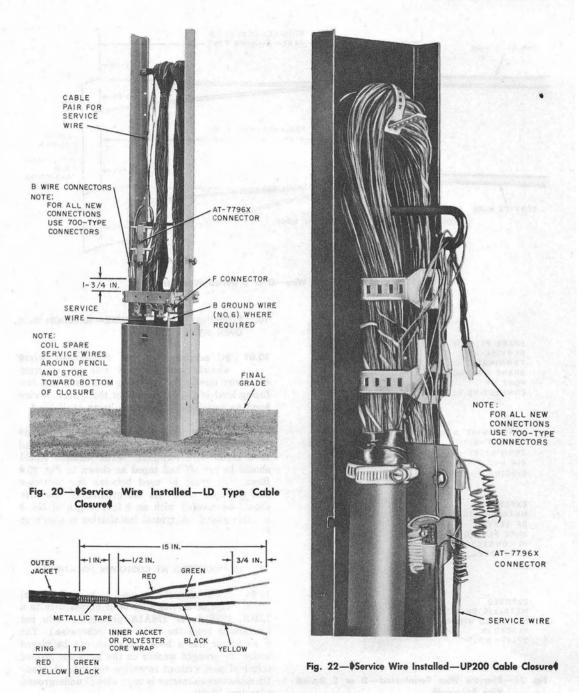
Fig. 21-Prepared Service Wire-UP200 Cable Closure
