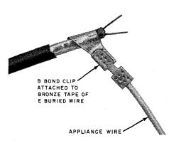
Fig. 27—♦Bonded Shield of E Buried Wire♥
