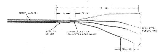
Fig. 15-Prepared Service Wire-E Cable Closure
