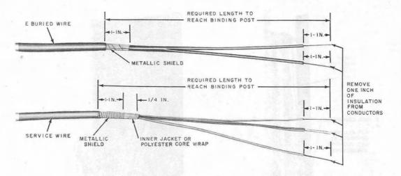
Fig. 23-Prepared Service Wire-D or E Buried Wire Terminal
