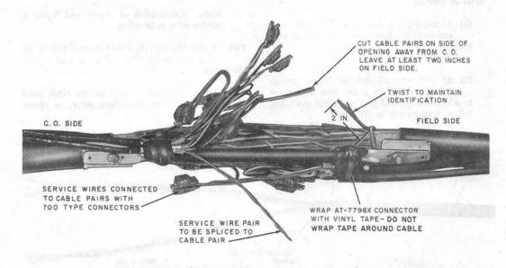
Fig. 5-DSplicing Cable Pairs-13-Type Closure
