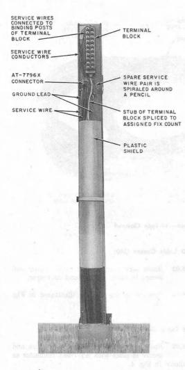
Fig. 8—\$Service Wires Terminated in RC4/72 Cable Closure J Cable Closure (MD)
