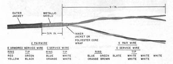
Fig. 3-Prepared Service Wire-13- or 14-Type Closure
