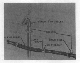
Fig. 10—Wires Crossing Power, Radio, or Television Wires on Masonry or Brick Surfaces
