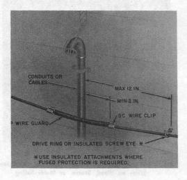
Fig. 11—Wires Crossing Cables, Conduits, Signal, or Ground Wires on Wood, Stucco, or Metal Siding
