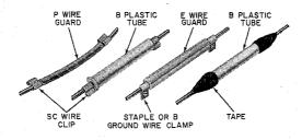
Fig. 1—Securing Plastic Tubes or E Wire Guard
