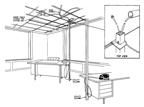
Fig. 10—Wiring Method With Utility Columns 4
