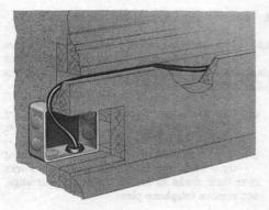
Fig. 5—Wiring From Conduit to Baseboards
