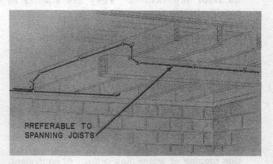
Fig. 8—Spanning Joist
