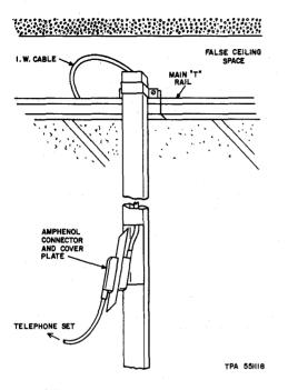
Fig. 11—Utility Column Installation 4
