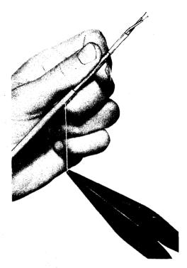
Fig. 6—Stripping SK Station Wire
