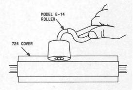
Fig. 14—Installing No. 724 Station Wire Cover
