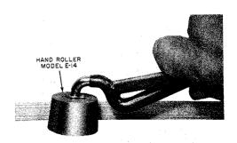
Fig. 3-Applying Roller to Wire Run
