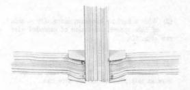
Fig. 9-Wire Tap Using No. 718 Tap
