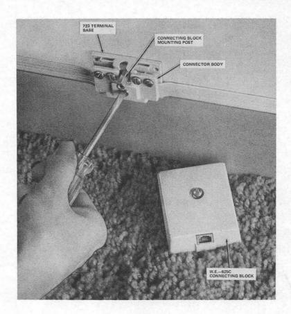
Fig. 12-No. 723 Terminal Base With W.E. 625C Connecting Block
