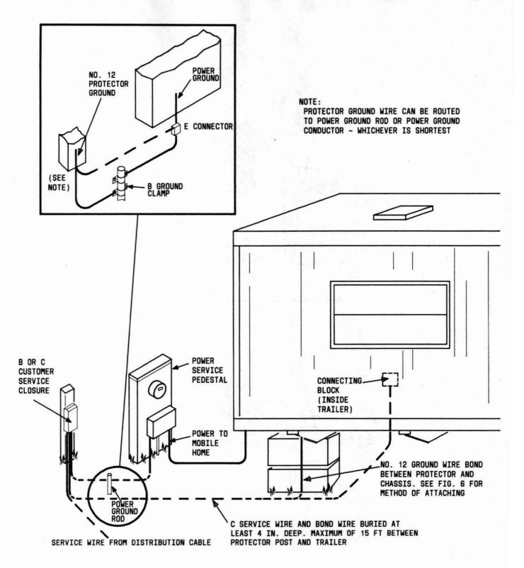
Fig. 5—Buried Service—Protector Located More Than 12 Inches From Mobile Home—Protector Grounded to Power Ground
