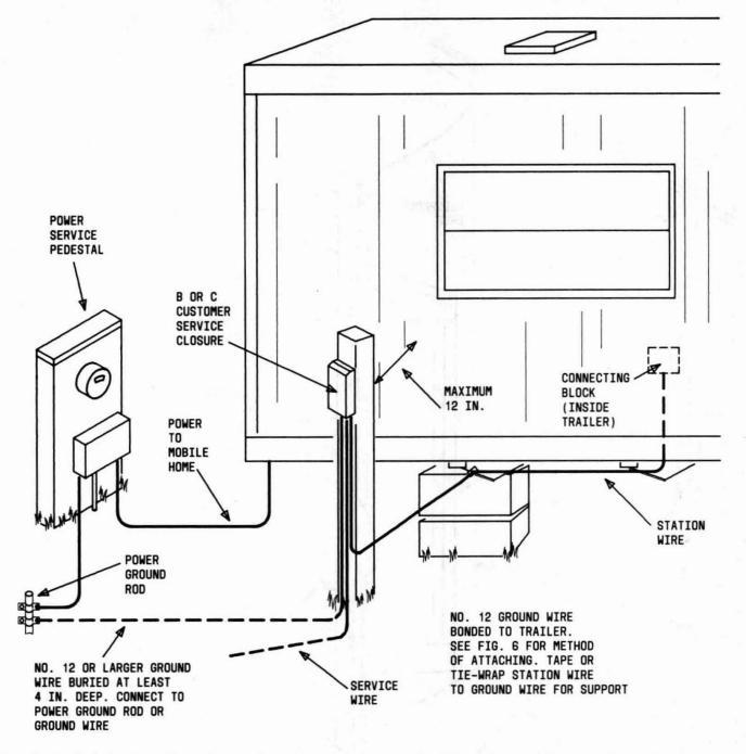
Fig. 3—Buried Service—Protector Located Witin 12 Inches of Mobile Home—Protector Grounded to Power Ground
