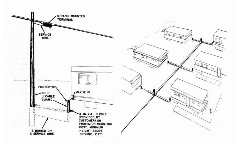
Fig. 1—Typical Buried Service Distribution
