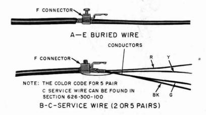
Fig. 8-F Connector on Service Wire
