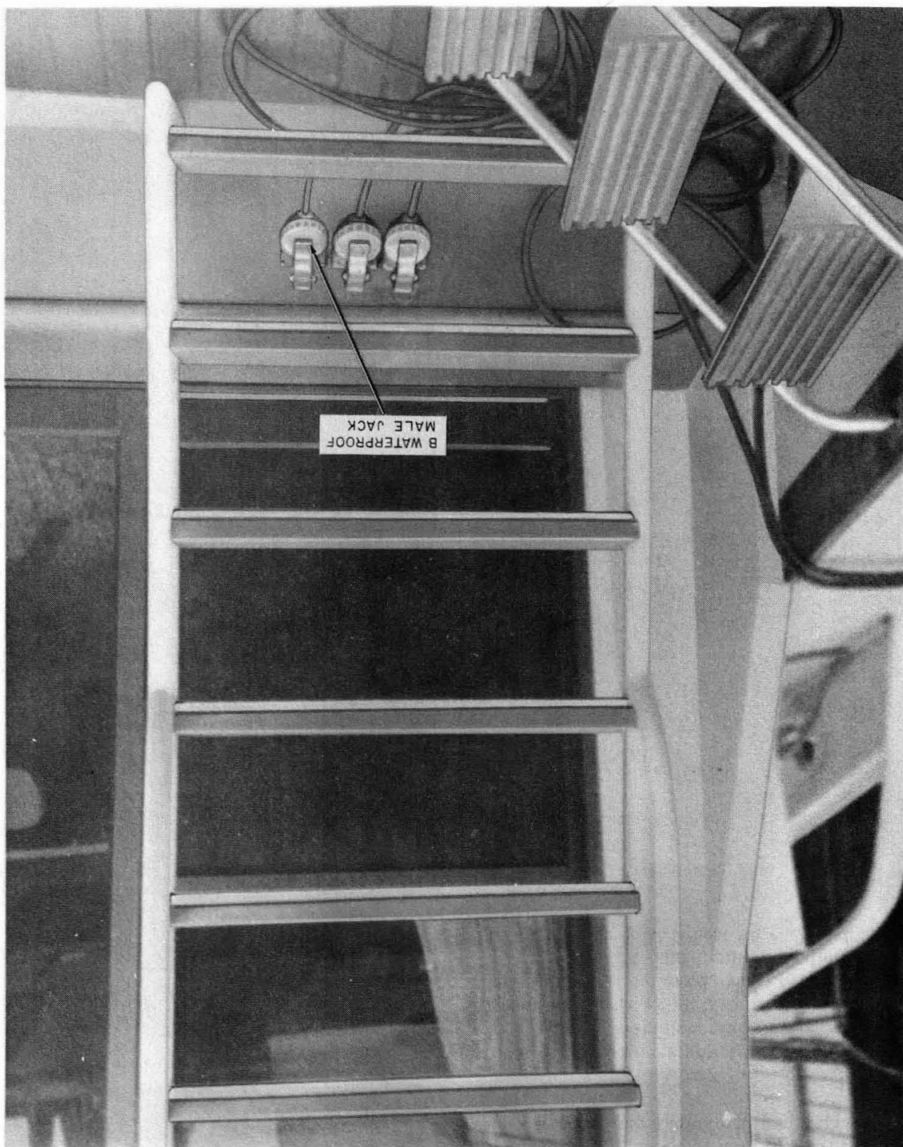
Fig. 21—Typical Boat Coaming B Waterproof Male Jack Installation
