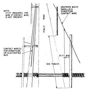
Fig. 3—Wire Crossing Railroad Tracks—Special Case
