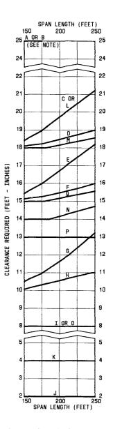
Fig. 24—Maintenance Clearances—Heavy Loading Area—Above or Alongside Thoroughfares or Obstructions—With Normal Sag
