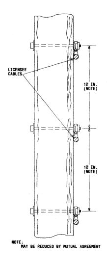
Fig. 13—Vertical Clearance Between Telephone Company and Licensee Cables
