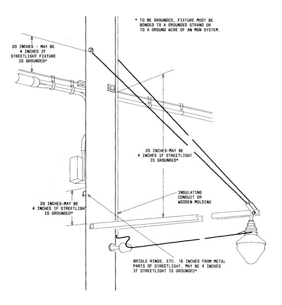
Fig. 10—Clearances of Drivehooks, Bridlewire Rings, or Brackets From Streetlight Fixture
