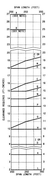
Fig. 23—Maintenance Clearances—Medium Loading Area—Above or Alongside Thoroughfares or Obstructions—With Minimum Sag
