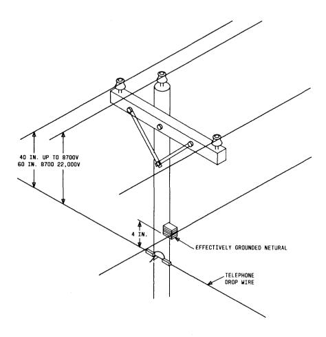
Fig. 14-Drop Wire Clearance on Common Crossing Pole
