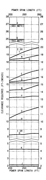
Fig. 20—Placing Clearances—Medium Loading Area—Above or Alongside Thoroughfares or Obstructions—With Mimimum Sag
