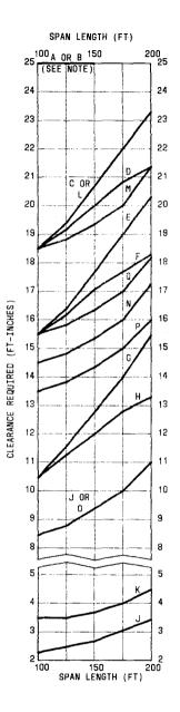
Fig. 22—Placing Clearances—Heavy Loading Area—Above or Alongside Thoroughfares or Obstructions—With Minimum Sag
