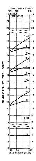
Fig. 25—Maintenance Clearances — Heavy Loading Area — Above or Alongside Thoroughfares or Obstructions—With Minimum Sag
