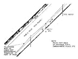
Fig. 8—Wire Running Along, But Not Overhanding, Nonrural Public Roads (Not Back of Obstruction)
