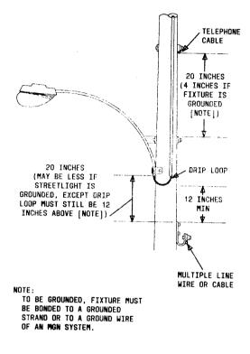
Fig. 9—Clearance From Streetlight Fixture Drip Loop Above Cable or Multiple Line Wire
