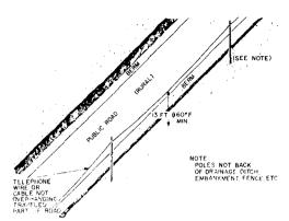
Fig. 7 -- Wire Running Along, But Not Overhanging, Publie Reads (Not Back of Obstruction)
