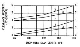
Fig. 19—Placing Clearances—Heavy Loading Area—Above, Below, or Alongside Electrical Facilities—With Normal and Minimum Sag
