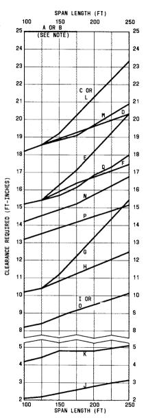
Fig. 21—Placing Clearances—Heavy Loading Area—Above or Alongside Thoroughfares or Obstructions—With Normal Sag
