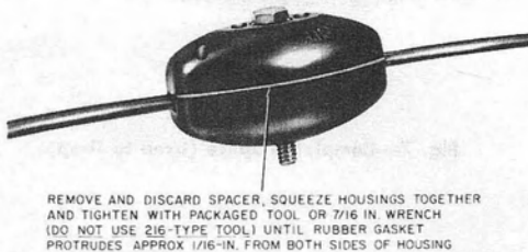
Fig. 8—Splicing Drop Wire with Amp Drop Wire Splice
