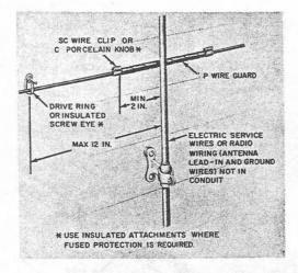
Fig. 11-Drop Wire Crossing Behind Foreign Wire
