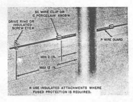
Fig. 10-Drop Wire Crossing Behind Pipe
