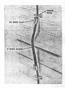
Fig. 3—Crossing Masonry Building Projection
