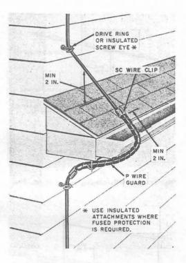
Fig. 9—Crossing Building Overhangs and Gutters
