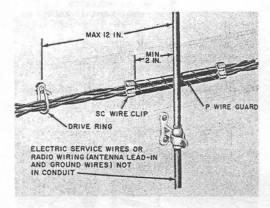
Fig. 12-Block Wire Crossing Behind Foreign Wire
