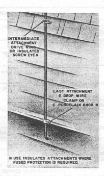
Fig. 4—Crossing Wood or Stucco on Wood Building
