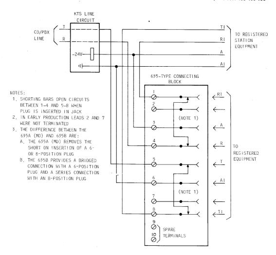
Fig. 6—Connections for USOC RJ34X
