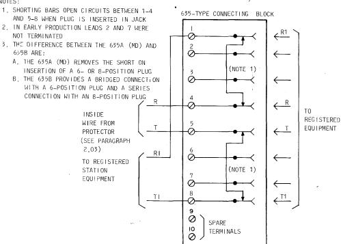
Fig. 4—Connections for USOC RJ32X
