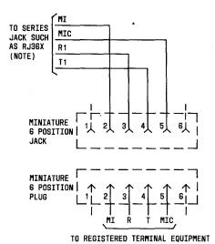
MI AND MIC LEADS ARE TYPICALLY WIRED TO AN RJ36X SERIES JACK WHICH CAN BE USED TO CONNECT AN EXCLUSION KEY TELEPHONE SET AHEAD OF THE DATA EQUIPMENT.
