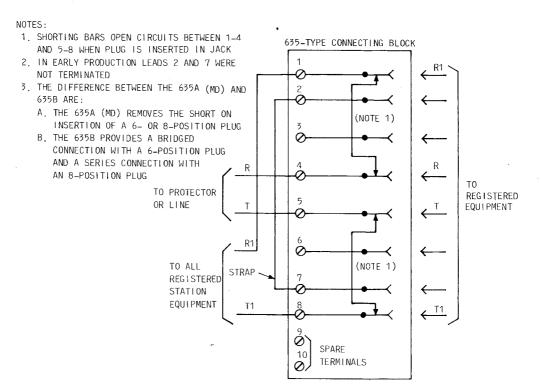
Fig. 10—Connections for USOC RJ38X
