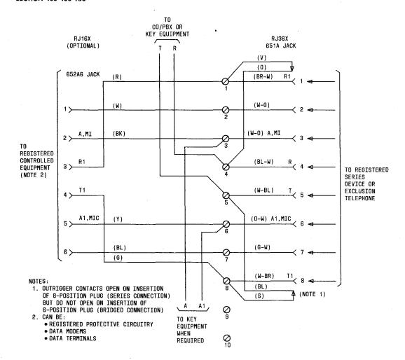
Fig. 1—Schematic Diagram, 635B Connecting Block (652A6 Jack for Controlled Station, Mounted in 635B Connecting Block Cover or Externally Mounted)
