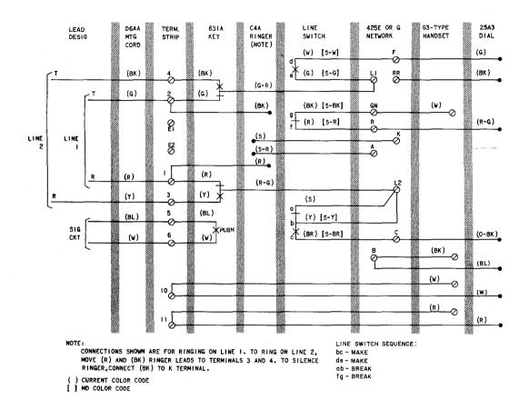
Fig. 1—♦1510F (MD) Telephone Set Connections With 25A3(MD) Dial, 2-Line Pickup and Signaling€
