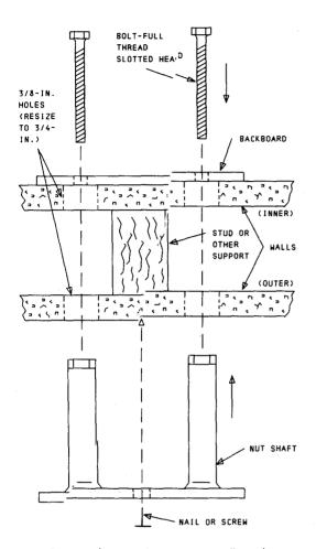
Fig. 10—₱Twin Bolt Fastener Installation €
