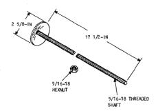
Fig. 11—▶Long-Bolt Fastener♦
