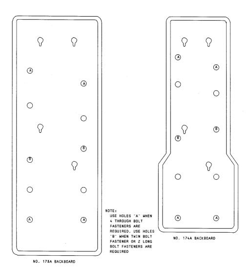
Fig. 9—▶Backboards Showing Mounting Holes♥
