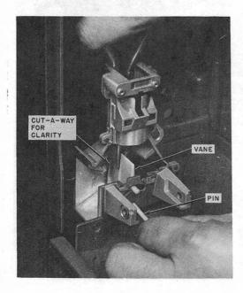
Fig. 4—Installing Pin in Vane
