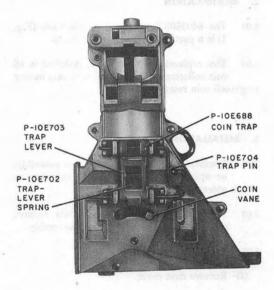
Fig. 2-Coin Trap and Trap-Lever Assembly
