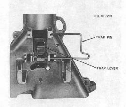
Fig. 6—Placing Trap-Lever Pin in Hopper
