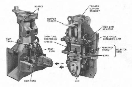
Fig. 8—Coin Hopper and Rear View of Coin Relay (Typical)
