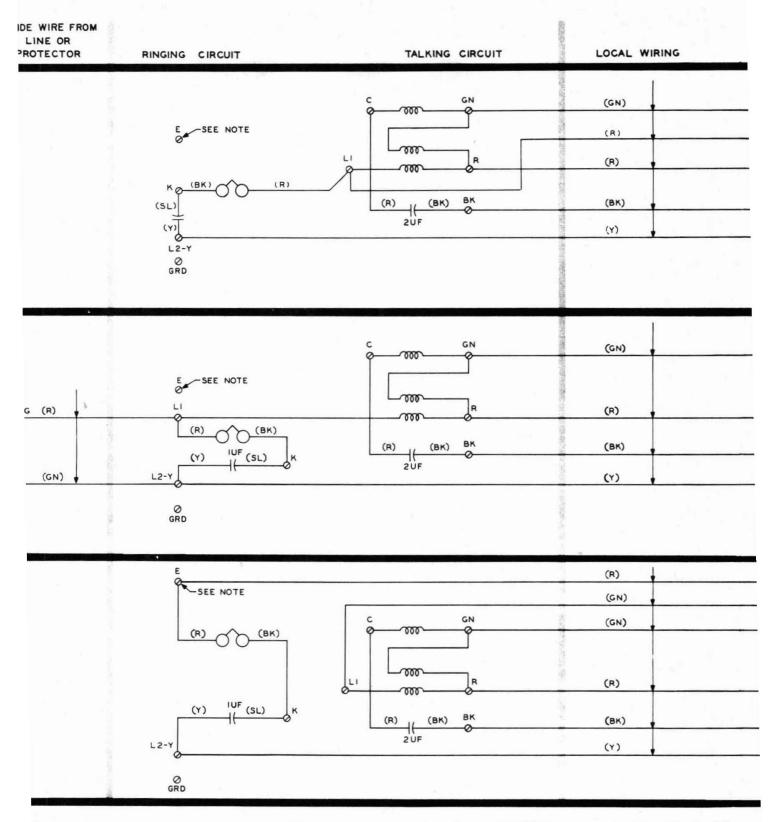
Nate: When an E terminal is not normally provided in subscriber sets, use D-161488 connector to connect local wiring to R ringer lead.
