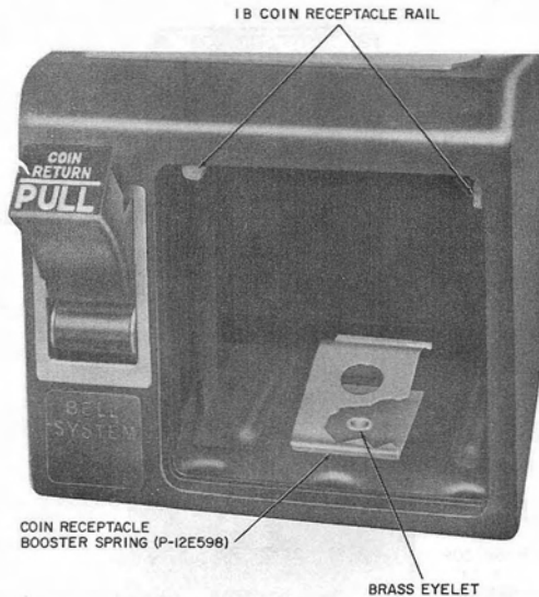
Fig. 6—Typical Lower Housing, Less Coin Receptacle Door
