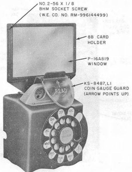
Fig. 9—Dial Type Coin Collector Equipped with Coin Gauge Guard
