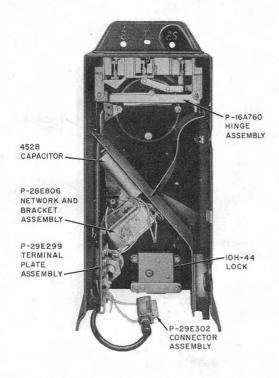
Fig. 11—Upper Housing With Gong Signal and Chute
