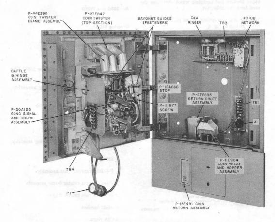
Fig. 5-235G or 1235G Coin Collectors-Interior View
