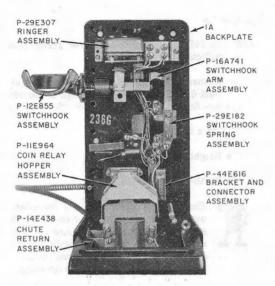
Fig. 9-P-89E100 Backplate Assembly
