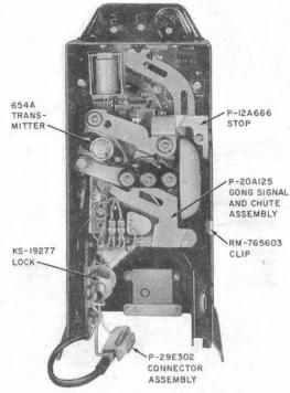
Fig. 10-P-89E000 Upper Housing Assembly
