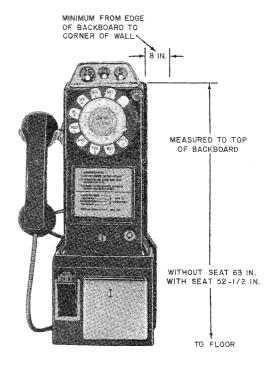
Fig. 13—Suggested Mounting Height and Clearance
