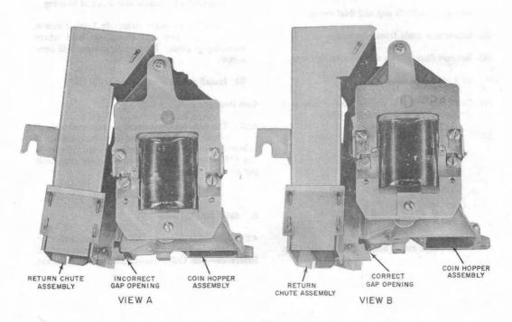
Fig. 19-Alignment of Return Chute Assembly
