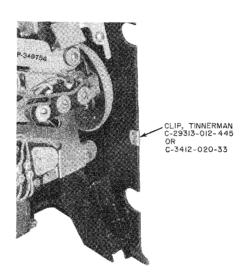
Fig. 16—Method of Grounding Upper Housing to Backplate
