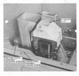
Fig. 18—Coin Relay and Return Chute Assembly
