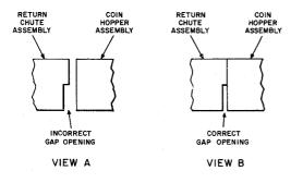
Fig. 20—Relative Position of Return Chute Assembly and Coin Hopper Assembly As Viewed Down Hopper Throat
