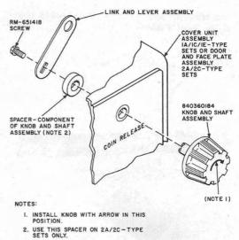
Fig. 62—Installation of 840360184 Knob and Shaft Assembly
