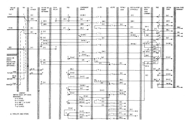
Fig. 71—1C2 or 2C2 Coin Telephone Set W/35T3A Dial—DTF Connections
