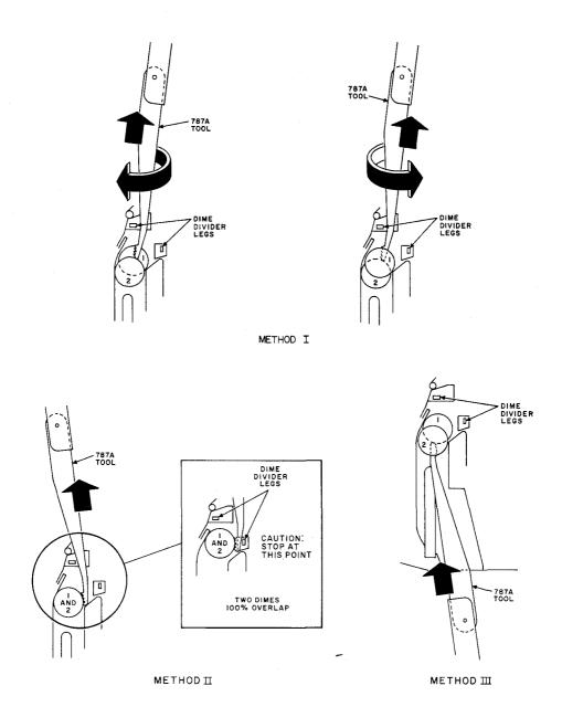
Fig. 43—Method for Removing Jammed Dimes From Chute
