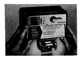
Fig. 20—Installing Instruction Cards in 1-Type Set (Typical)
