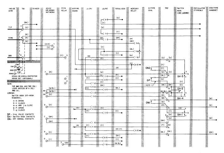
Fig. 64-1A1 of 2A1 Coin Telephone Set-Connections
