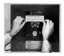
Fig. 25—Installing Instruction Card in 2-Type Set
