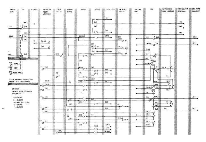
Fig. 66—1A2 or 2A2 Coin Telephone Set W/70-Type Dial—Connections
