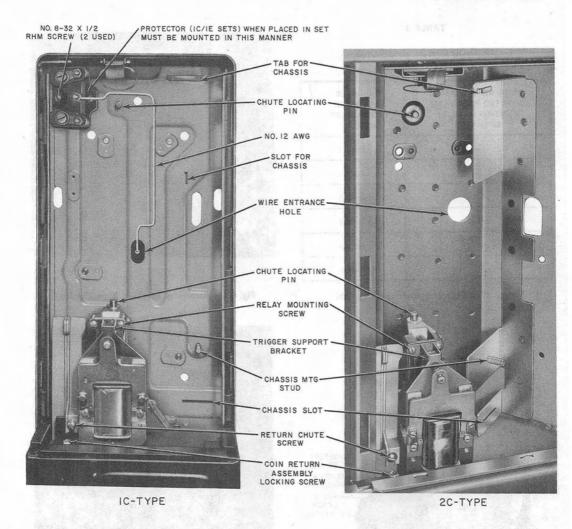
Fig. 13—Housing and Mounting Plate Assembly
