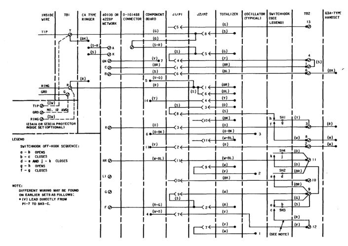
Fig. 74—1E3 Coin Telephone Set—Connections
