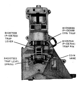
Fig. 47—Coin Trap and Trap Level Assembly
