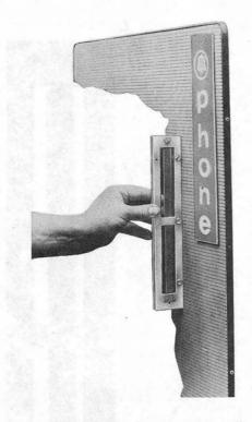
Fig. 8—KS-22473 Leveling Device Being Used to Check Wall and Backboard Alignment
