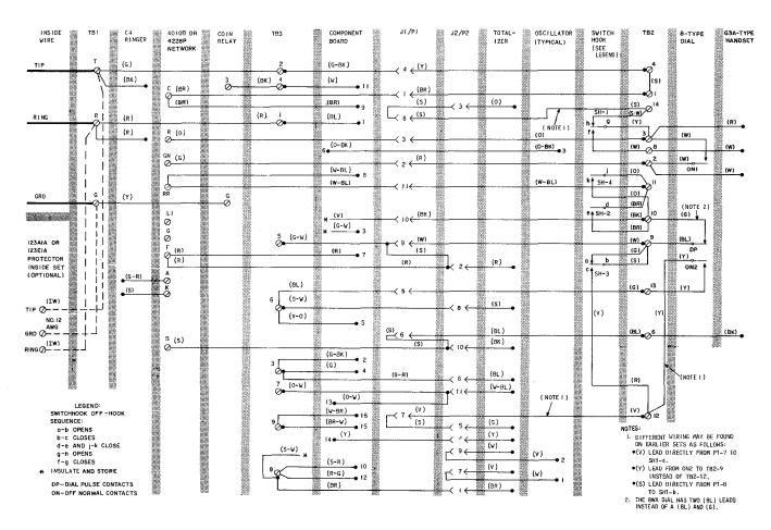
Fig. 68—1C1 or 2C1 Coin Telephone Set—DTF Connections
