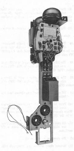
Fig. 19—30B Coin Chassis—For Use in 1E-Type Sets
