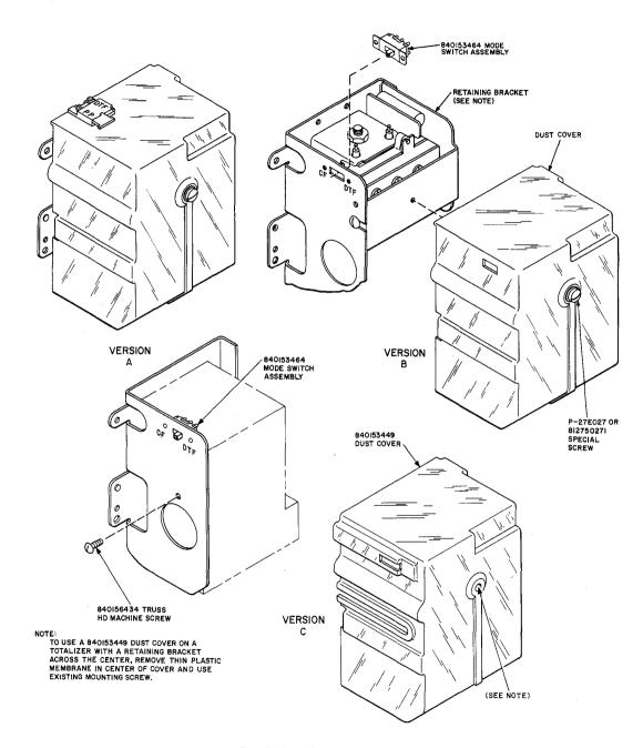
Fig. 5—Partial View of Totalizer
