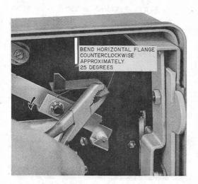
Fig. 61—Bending Chute Guide (Limit Stop)
