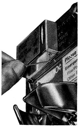
Fig. 57—Setscrew Adjustment
