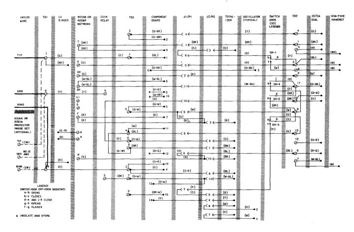
Fig. 69—1C2 or 2C2 Coin Telephone Set W/35T3A Dial—CF Connections
