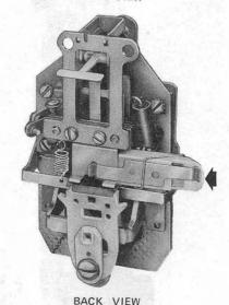
Fig. 36—Bias Margin Gauge in Position for Collect Test
