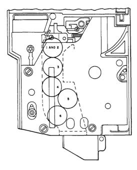
Fig. 42—Lower Portion of Coin Chute With Six Dimes
