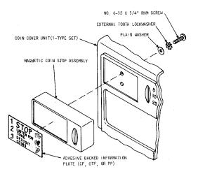
Fig. 56—Installation of the D-180848 Kit of Parts (Magnetic Coin Stop)
