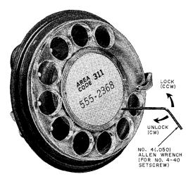
Fig. 26—Installing Fingerwheel on 8U (MD), 8W (MD), or 8WA Dial
