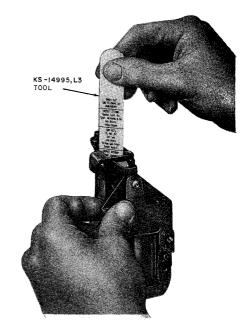
Fig. 38—Trap and Vane Release Test
