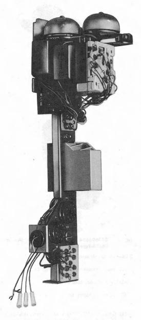
Fig. 18—31A Coin Chassis—For Use in 1C/2C-Type Sets
