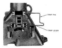
Fig. 48-Placing Trap Lever Pin on Hopper
