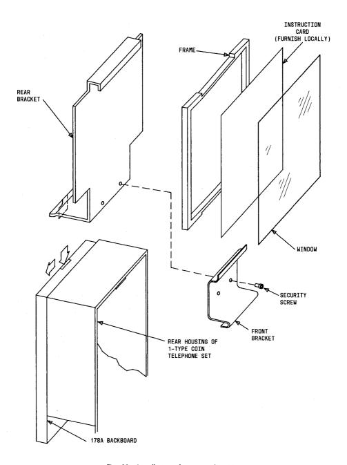
Fig. 23-Installation of 11A Card Holder
