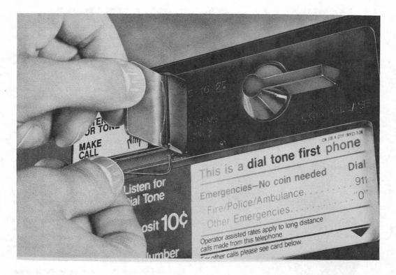
Fig. 59—KS-22551 Gauge Being Used to Adjust No. 4-40 Setscrew
