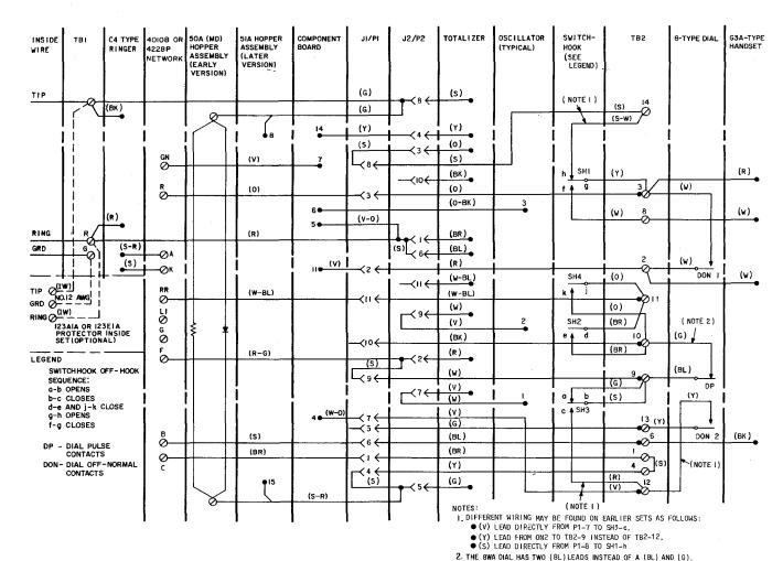
Fig. 73-1E1 Coin Telephone Set-Connections
