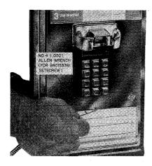
Fig. 21—Securing Instruction Card (Typical)
