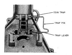
Fig. 49-Placing Coin Trap in Hopper
