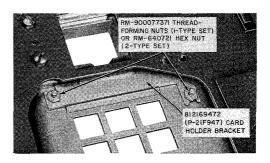
Fig. 29—Card Holder Bracket Installed in TOUCH-TONE
