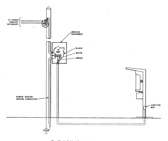
Fig. 10-Individual Power Source to Mounting
