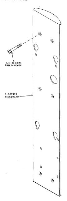
Fig. 4—KS-19206, List 7 Coin Telephone Set Installation Kit
