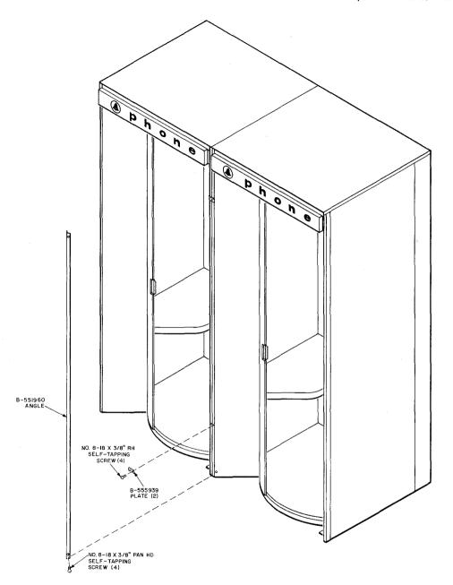
Fig. 5—KS-19206, List 10 Multiple Installation Kit (Items Identified)
