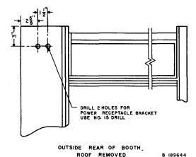
Fig. 26—Holes for Mounting Receptacle Bracket
