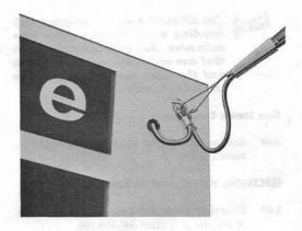
Fig. 15—Drop Wire Hook For First Attachment
