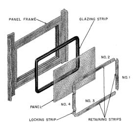
Fig. 24—Assembly of Side or Rear Panels
