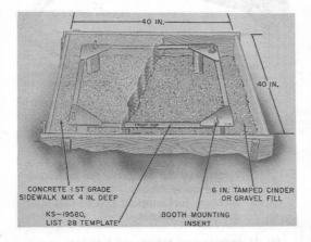
Fig. 14—Concrete Base Preparation with KS-19580, **List 28 Template**
