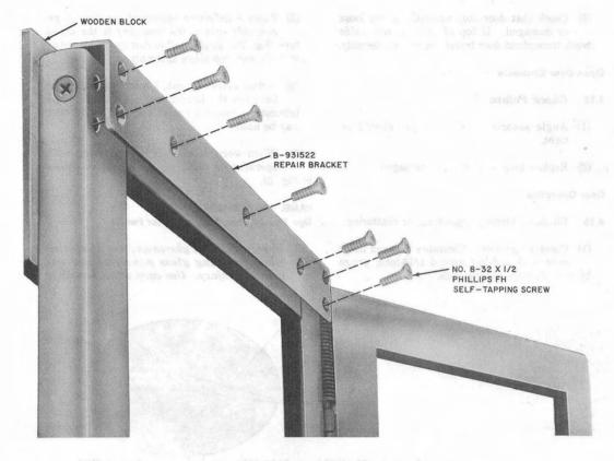
Fig. 20—Installation of Door Repair Bracket
