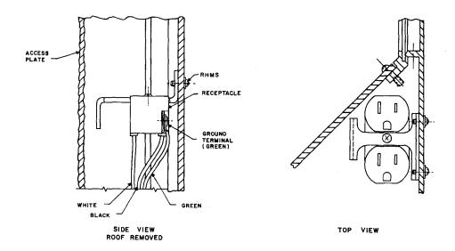
Fig. 27—Location and Wiring of Receptacle
