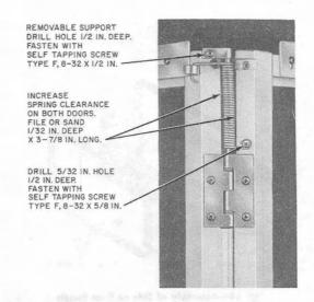
Fig. 22—Installation of Top Hinge Assembly
