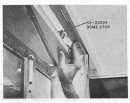
Fig. 5—Releasing Dome Stop
