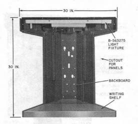
Fig. 8—KS-19426, List 1 Housing Less Light Shield
