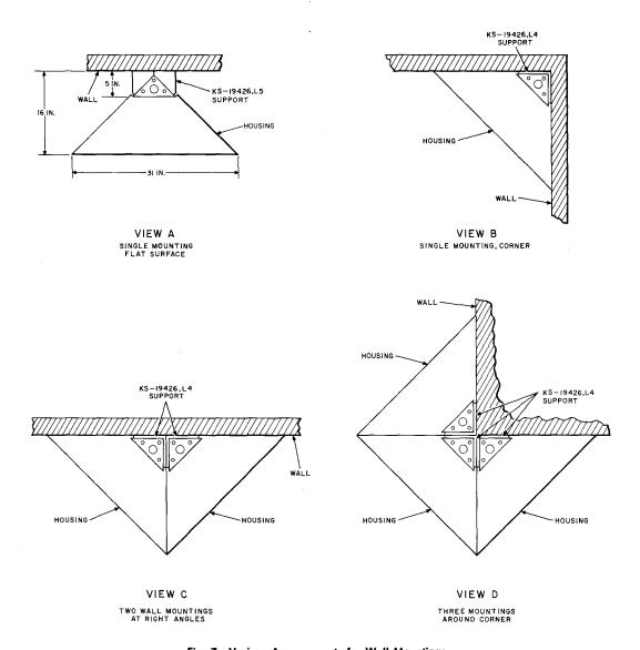
Fig. 7-Various Arrangements for Wall Mountings
