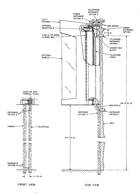
Fig. 22—Installation Requirements for Wall Mountings
