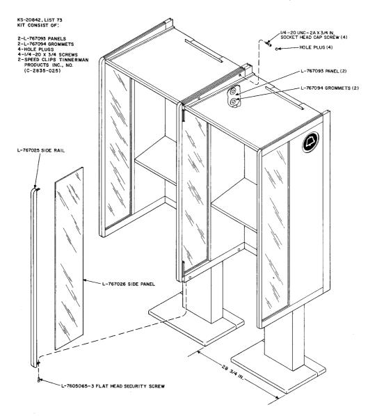
Fig. 33-Two List 32 Housings Side-By-Side
