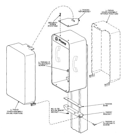
Fig. 45—KS-20842, List 75 Cover Assembly—Installation Procedure
