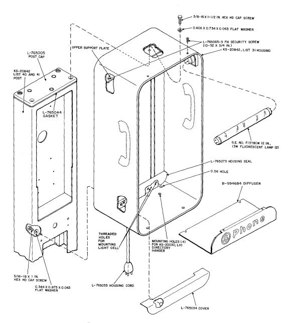
Fig. 29—Installation of List 31 Housing on Post
