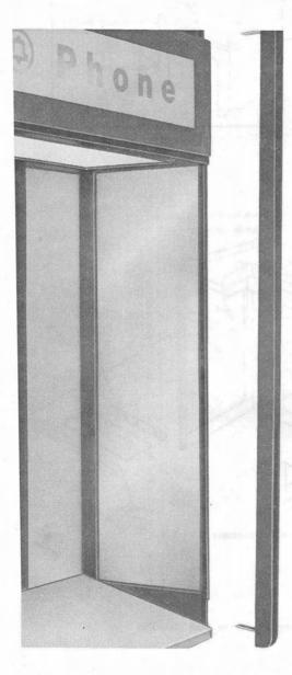
Fig. 27—Removal of Front Vertical Rail from List 35 Housing
