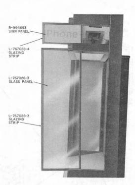
Fig. 38—Removal of Glass Panel and Sign Panel from List 35 Housing
