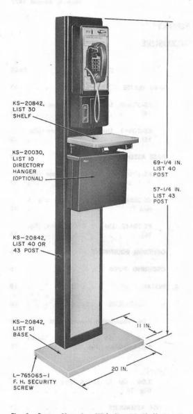
Fig. 1—Sentry Mounting With List 30 Shelf (List 2 or 37 Arrangement)
