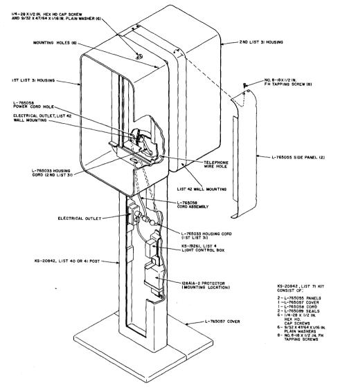
Fig. 31—Installation of Two List 31 Housings, Back-to-Back On One Post
