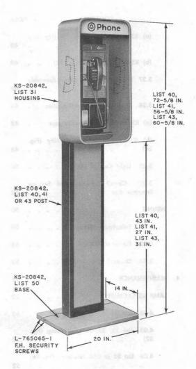
Fig. 2—List 31 Housing—Post Mounted (List 5, 9, or 23 Arrangement)
