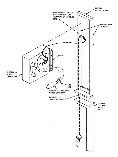
Fig. 42-Installation of KS-20135 Sign
