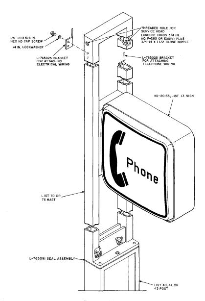
Fig. 41—Installing List 70 Mast on Post
