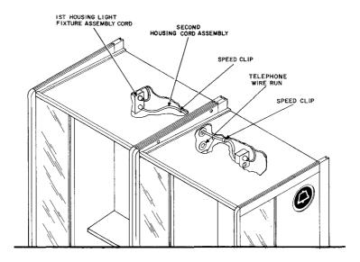
Fig. 35—Wire-Runs Between Two Walk-in Housings Side-By-Side
