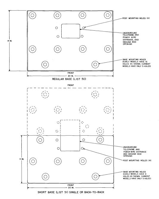
Fig. 25—Layout of Holes in List 50 and List 51 Bases, With Cover(s) Removed
