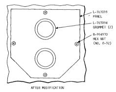
Fig. 34—Replacing Bell Symbol Sign With Panel
