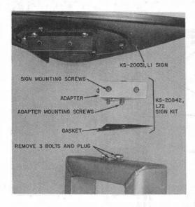
Fig. 43—Installation of KS-20031, List 1 Sign
