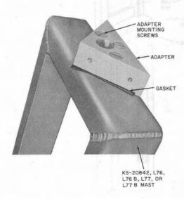
Fig. 44—Installation of KS-20842, List 72 Sign Kit
