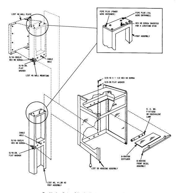
Fig. 36—Installation of List 35 Housing on Post or Wall Mounting
