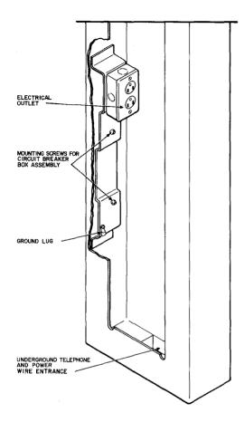
Fig. 30—Outlet for Terminating Electrical Service and Optional KS-19426, List 17 Circuits Breaker Box Mounting Location
