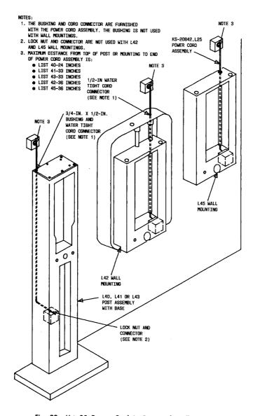
Fig. 22—List 25 Power Cord in Post and Wall Mountings
