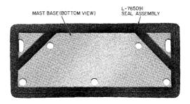
Fig. 40—Bottom View of Mast Showing Correct Position of Seal
