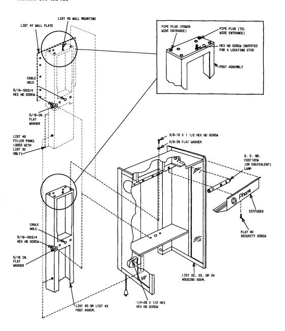
Fig. 32—Installation of List 32, 33 or 34 Housing on Post or Wall Mounting
