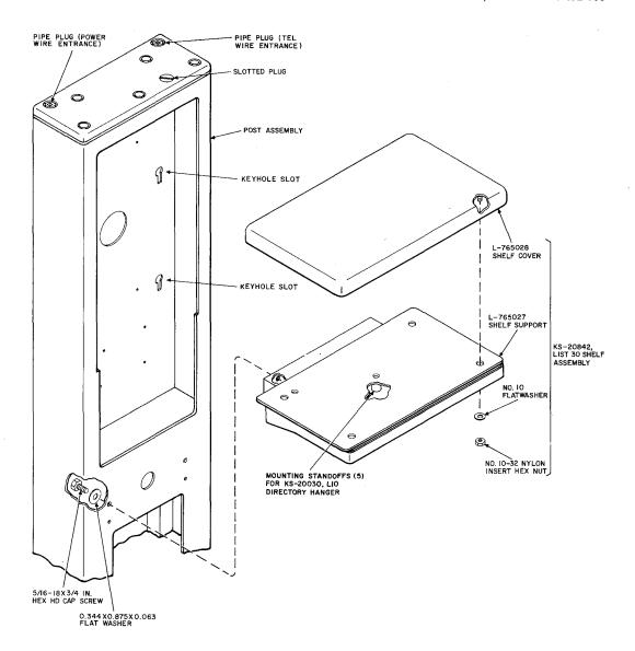
Fig. 28—Installation of List 30 Shelf on Post
