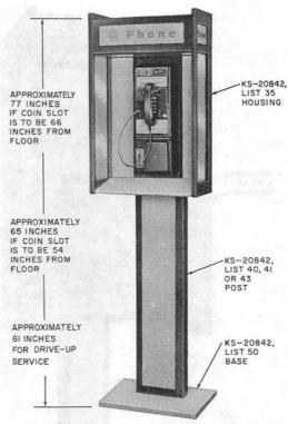
Fig. 10—List 35 Housing—Post Mounted (List 82, 85, or 90 Arrangement)
