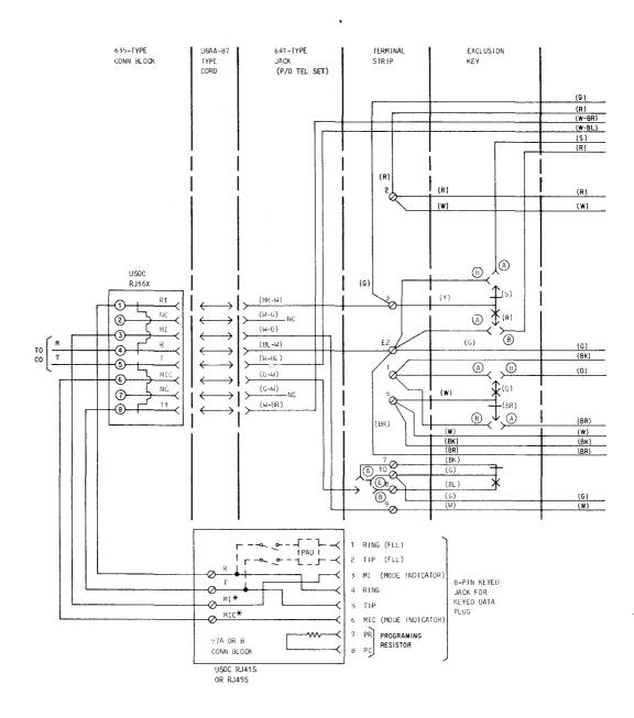
Fig. 14—2503CM Telephone Set—Registration Jack Connections (Sheet 1 of 2)
