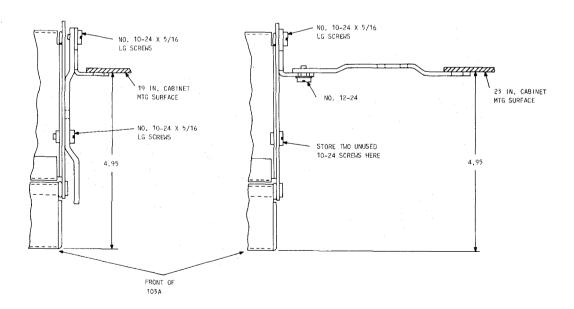
Fig. 16—103A Apparatus Mounting Brackets
