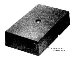
Fig. 2-97B Connecting Block
