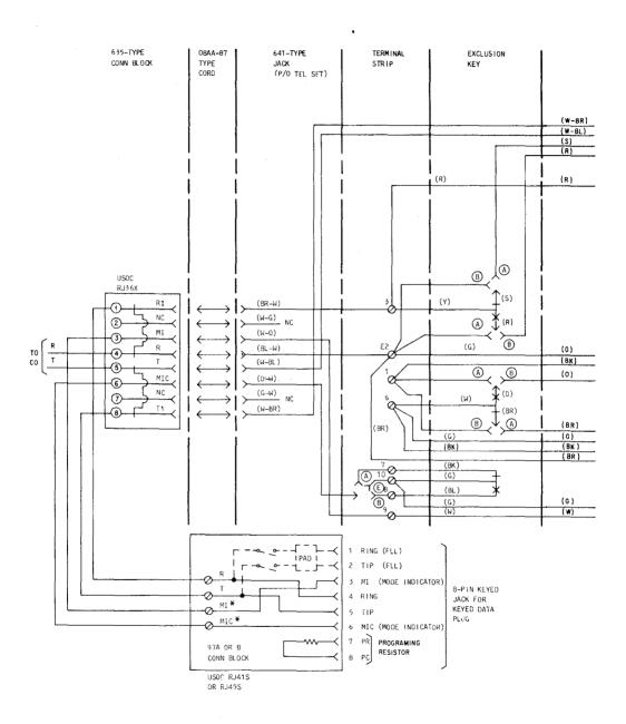
Fig. 13—503CM Telephone Set—Registration Jack Connections (Sheet 1 of 2)
