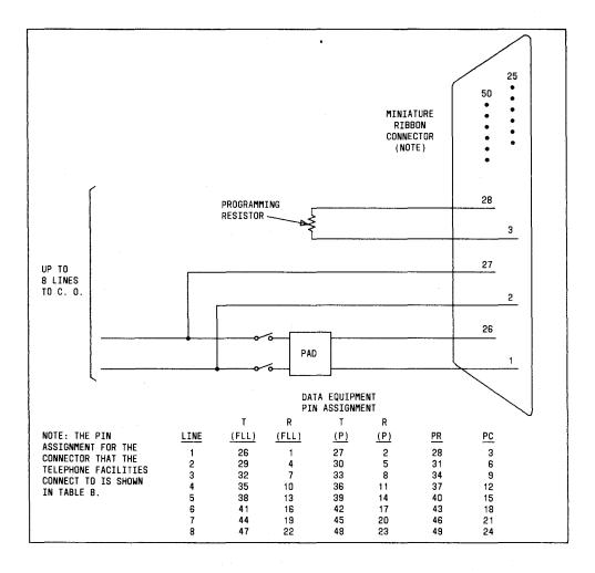
Fig. 11—USOC RJ26X, Schematic
