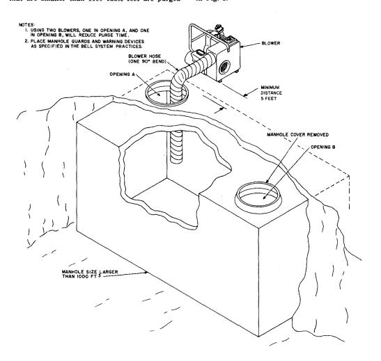
Fig. 1—Typical Setup for Purging Large Conventional Manholes
