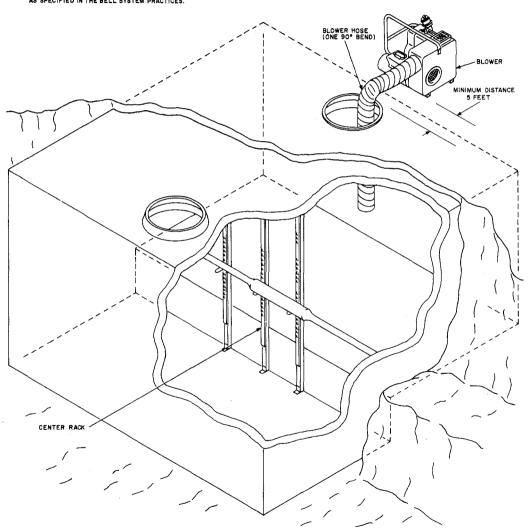
Fig. 2—Typical Setup for Purging Irregular Shape Manholes
