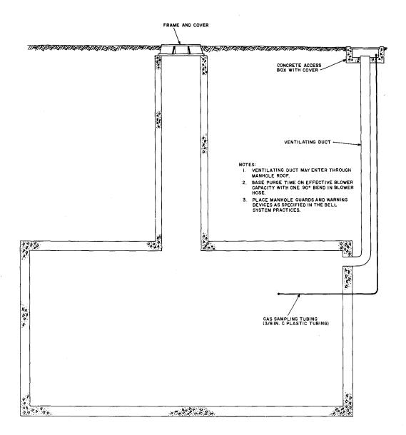
Fig. 7—Deep Neck Manhole With Permanent Ventilating Duct Installed Adjacent to Manhole
