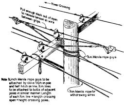
(j) Cut line wire about one foot from crossarm on crossing side. Untie 1/2 inch manila rope line from arm and loop end of wire over crossing through the eye of this line and serve the wire about itself securely. This wire should be drawn tightly enough so that excess sag will not develop when grips are removed.
