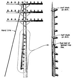
The handline should be passed through a rope lashing placed near the top of the pole for removal of top arm.
