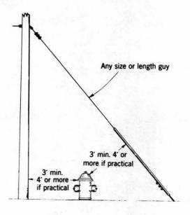
Fig. 30—Telephone Cable on Guys Above or Alongside Fire Hydrants, Signal Pedestals
