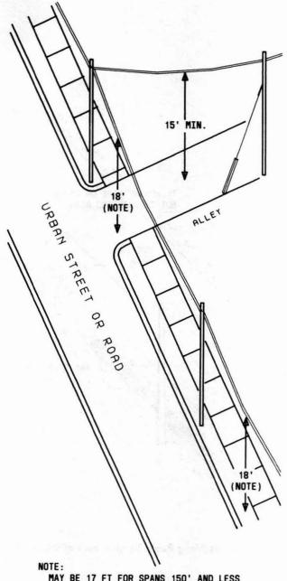
MAY BE 17 FT FOR SPANS 150' AND LESS CABLE SUPPORTED ON MESSENGER. DOES NOT APPLY TO ARTERIAL ROADS
