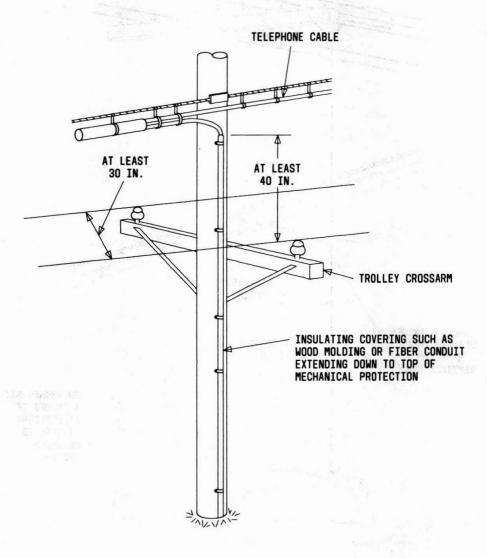
Fig. 20—Clearances Between Trolley Crossarms and Telephone Cable
