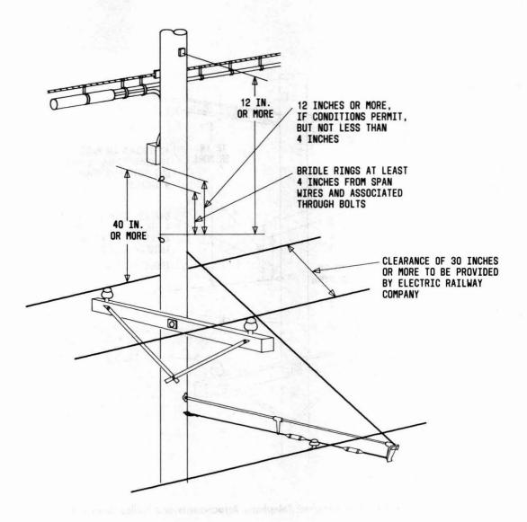
Fig. 21—Clearances Between Telephone Attachments and Trolley Wire Attachments
