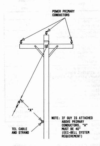
Fig. 23—Clearance Between Power Guy and Telephone Cable and Strand
