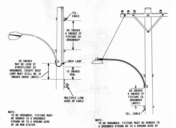
Fig. 16—Clearance From Streetlight Fixture Drip Loop Above Cable or Multiple Line Wire
