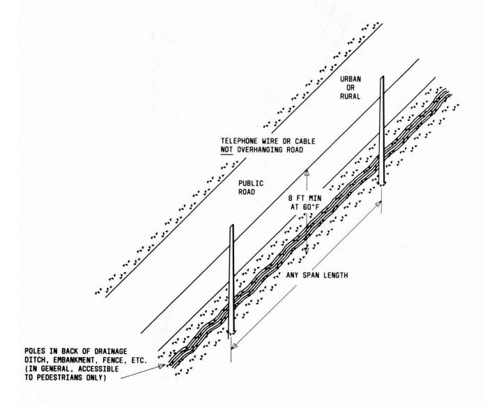
Fig. 7—Running Along Public Roads—Back of Ditches, Etc.
