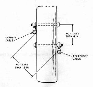
Fig. 25—Diagonal Clearance Between Licensee and Telephone Cables
