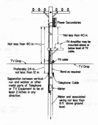
Fig. 29—Clearances on Joint-Use Pole With TV Amplifier and Meter Mounted on Pole
