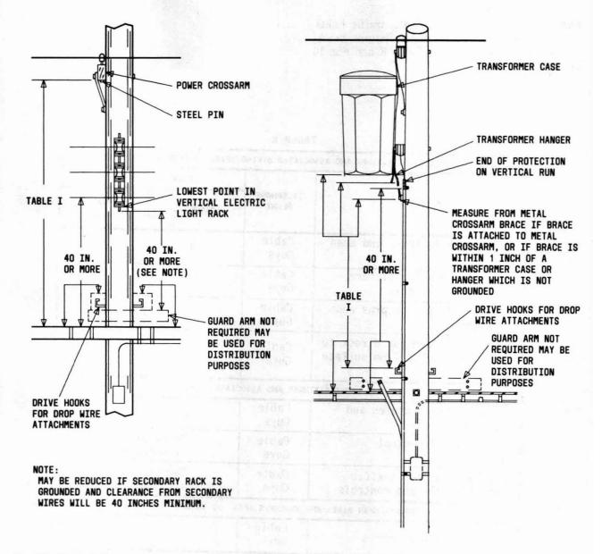
Fig. 14—Vertical Clearances Between Cable and Power Attachments
