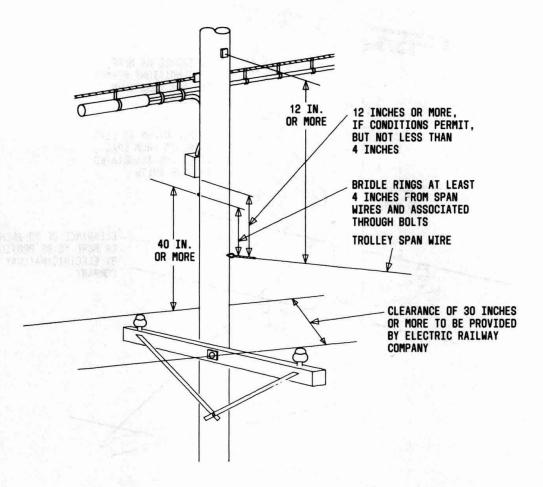
Fig. 22—Clearances Between Telephone Attachments and Trolley Span Wire
