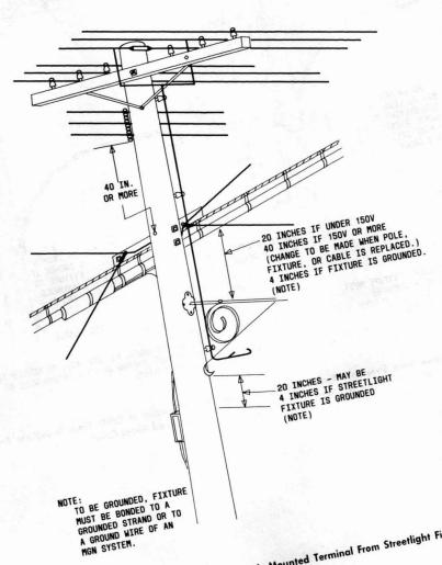
Fig. 18—Clearances of Cable and Pole-Mounted Terminal From Streetlight Fixture
