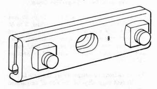
Fig. 5—B Cable Suspension Clamp
