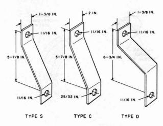
Fig. 7—Reinforcing Straps
