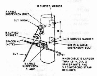
Fig. 16—6M or 6.6M Suspension Strand—Pull Less Than 10 Feet
