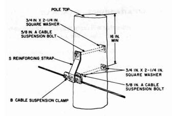
Fig. 15—Pole Attachment with Reinforcing Strap
