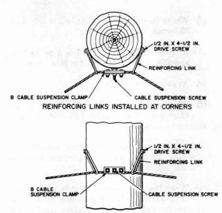
REINFORCING LINKS INSTALLED AT DOWNWARD CHANGES IN GRADE
