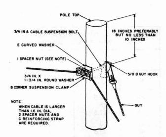
Fig. 19—6M or 6.6M Suspension Strand-Pull Away
