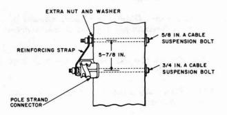
Fig. 10—Nut and Washer Used to Space Reinforcing
