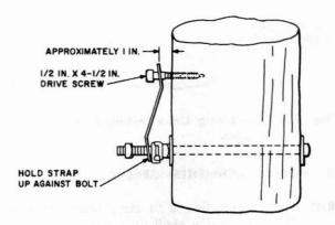
Fig. 8—Installing Reinforcing Strap Using Drive Screw
