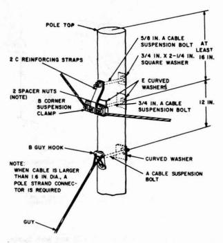
Fig. 20—10M Suspension Strand with Spacer
