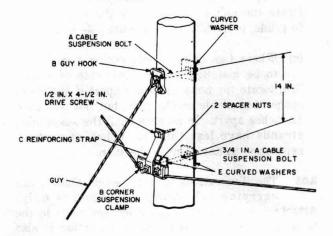
Fig. 17—6M or 6.6M Suspension Strand with Spacer Nuts—Pull Toward Pole—10 Feet to 50 Feet
