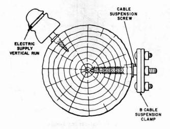
Fig. 4—Installed Cable Suspension Screw
