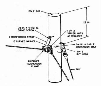
Fig. 21—10M Suspension Strand—Pull Away From Pole—5 Feet to 50 Feet
