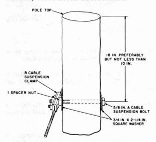
Fig. 13—Pole Attachment for 6M or 6.6M Suspension Strand With No Reinforcing Strap
