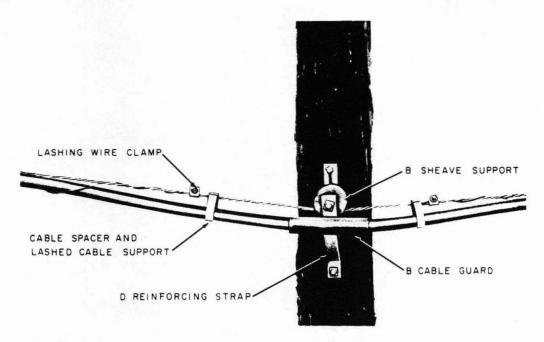
Fig. 25—B Sheave Support and D Reinforcing Strap Used to Support Strand and Cable at a Grade Change
