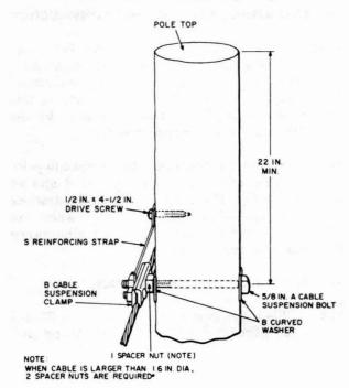
Fig. 14—Pole Attachment with Reinforcing Strap
