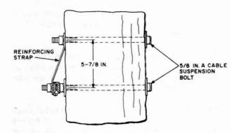
Fig. 9—Installing Reinforcing Strap Using Bolt
