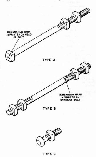
Fig. 1—Cable Suspension Bolts
