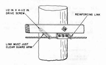
Fig. 12—Reinforcing Links Installed at Guard Arm Location
