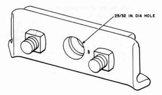
Fig. 6—B Corner Suspension Clamp
