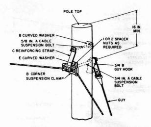
Fig. 24—25M Suspension Strand—Pull Away From Pole—5 Feet to 40 Feet
