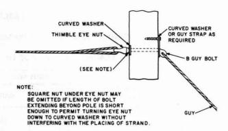
Fig. 2—B Guy Bolt and Associated Hardware Installed
