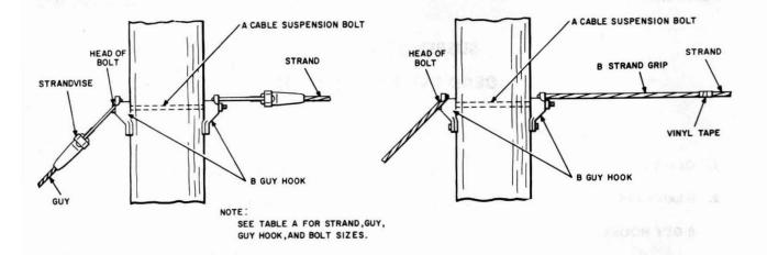
Fig. 1-Installed B Guy Hooks and Associated Hardware
