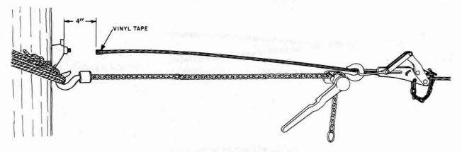
Fig. 5-Tensioned Strand
