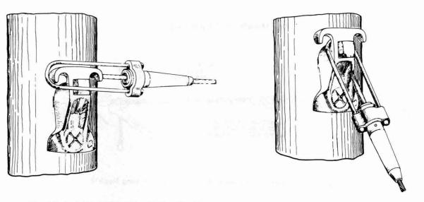
Fig. 14—Installing Strandvise (B Guy Hook)
