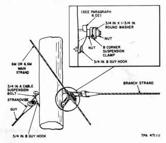
Fig. 22—Branch Strand Termination—6M or 6.6M
