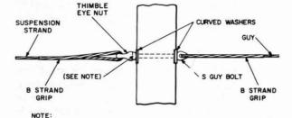
SQUARE NUT UNDER EYE NUT MAY BE OMITTED IF LENGTH OF BOLT EXTENDING BEYOND POLE IS SHORT ENOUGH TO PERMIT TURNING EYE NUT DOWN TO CURVED WASHER WITHOUT INTERFERING WITH THE PLACING OF STRAND.
