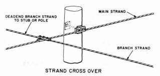
Fig. 26—Branch Cable Strand Termination
