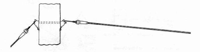
Fig. 19—♦Completed Installation (Strandvise)♦
