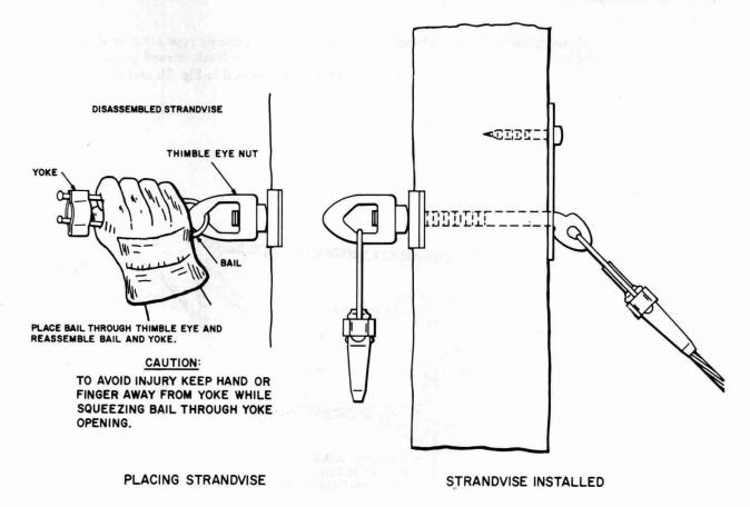
Fig. 13—Installing Strandvise (Thimble Eye Nut)
