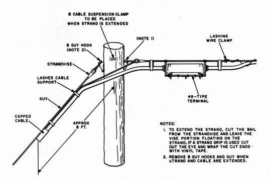
Fig. 29—DExtending Strand at Dead-end Termination
