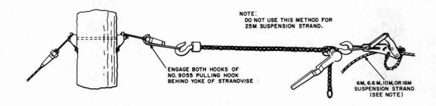
Fig. 17-Strand Attachment (Reliable No. 9055 Strand Pulling Hook)
