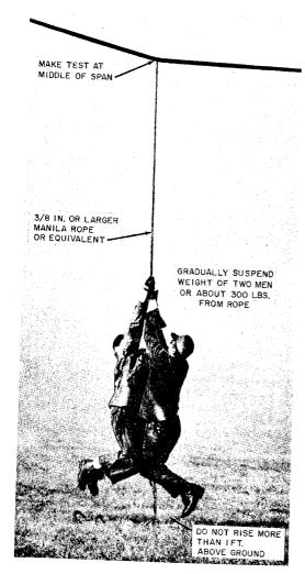
Fig. 2—Testing Strand Prior to Placing Aerial Platform or Cable Car
