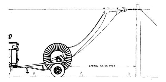
Figure 2. Positioning Cable Reel
