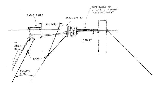
NOTE: Approximately 4 feet for metallic conductor cable, and 6 feet for optical cable
