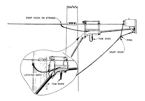
Figure 5. Transferring Cable Guide
