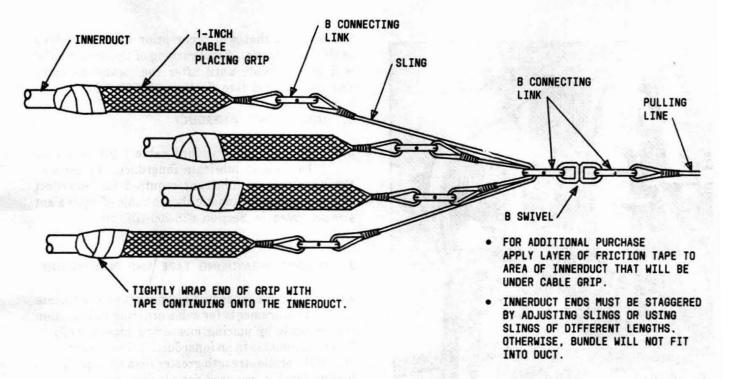
Fig. 2—Method of Attaching Pulling Line to Innerduct
