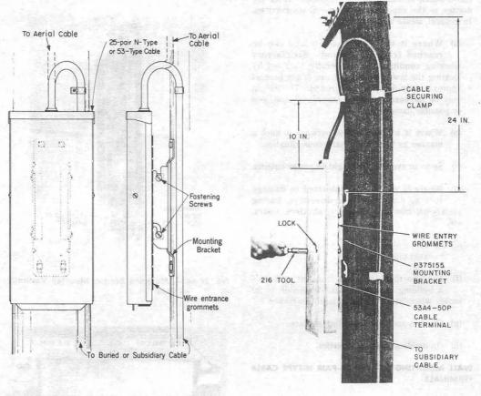
Fig. 26—Installing Cable Terminal on Pole Mounting Bracket
