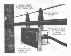
Fig. 14—10- or 16-Pair N-Type Cable Terminal Installed
