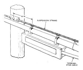
Fig. 16—Strand Mounted Terminal Installed On Ring Supported Cable—Cable/Strand Space Greater than 2 1/2-Inches
