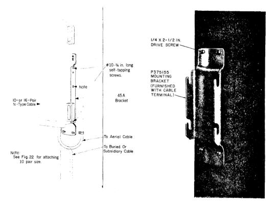
Fig. 24—10- or 16-Pair N-Type Cable Terminal Attached To Mounting Bracket
