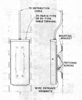
Fig. 37—Installing Terminal on Mounting Bracket
