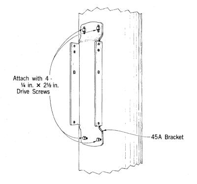
Fig. 23—Attaching 45A Mounting Bracket To Pole
