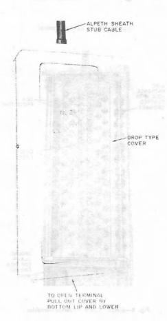
Fig. 11—Opening Cover of 25-Pair N-Type Cable Terminals
