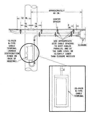
Fig. 13-Placing Pole-Mounted Cable Terminal
