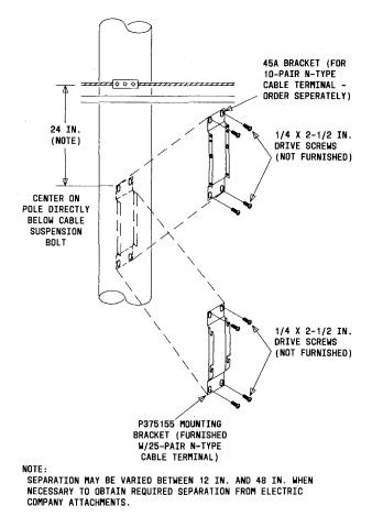
Fig. 12—Locating Mounting Bracket
