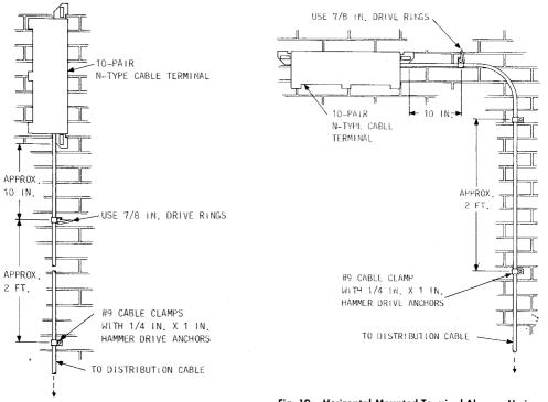
Fig. 18—Vertical-Mounted Terminal Above a Horizontal Cable Run
