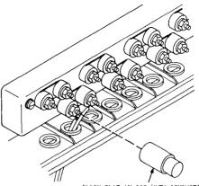
ALIGN SLIT IN CAP WITH CONDUCTOR AND WITHOUT TWISTING PUSH DOWN UNTIL SKIRT OF CAP CONTACTS PEDESTAL.
