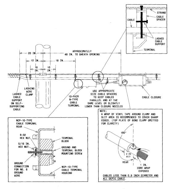
Fig. 10-Placing Strand-Mounted Cable Terminal
