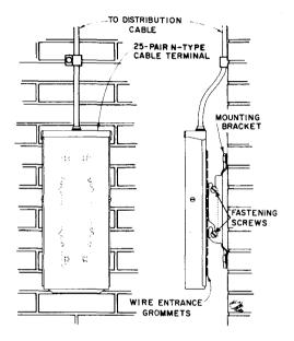
Fig. 21—Installing Terminal on Mounting Bracket
