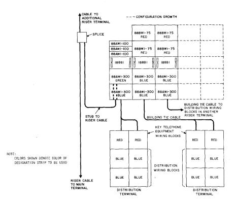
Fig. 7—Block Diagram Showing Riser Terminal Serving Two Distribution Terminals
